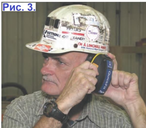
Fig. 3. Worker adjusted the volume control on the QuickFit device to set his hearing threshold before inserting an earplug.
