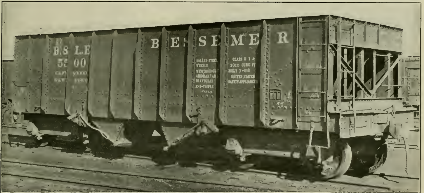
Fig. 1.—Steel Hopper Car 20 Years Old; 80,000 lb. Capacity; Light Weight, 41,900 lb.
