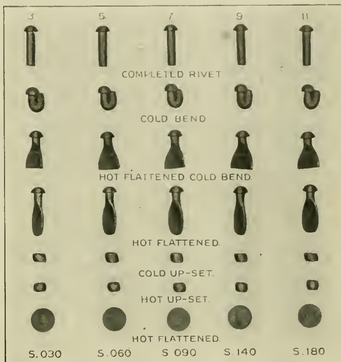
Fig. 1—Results of Hot and Cold Bending and Flattening Tests
