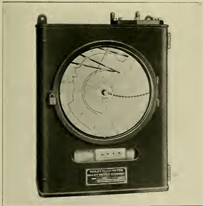
Bailey Fluid Meter with Pressure and Temperature Recording Pens
