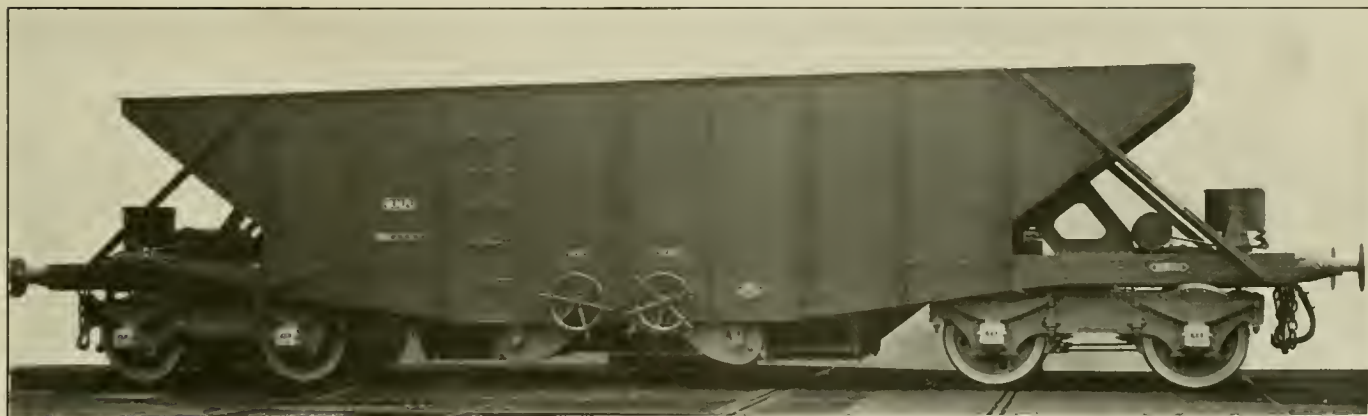
Steel Hopper Car Built in England for the Bengal-Nagpur Railway
