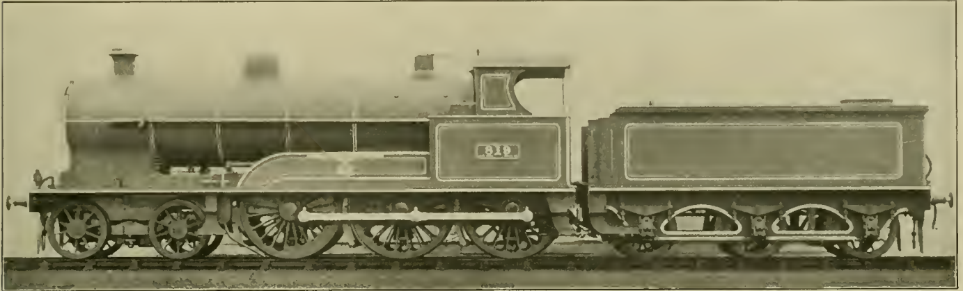
Six-Coupled, Two-Cylinder, Superheater Locomotive, London & North Western
