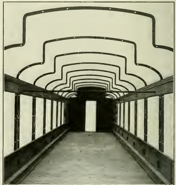
Interior of the Steel Frame; Canadian Northern Sleeping Cars
