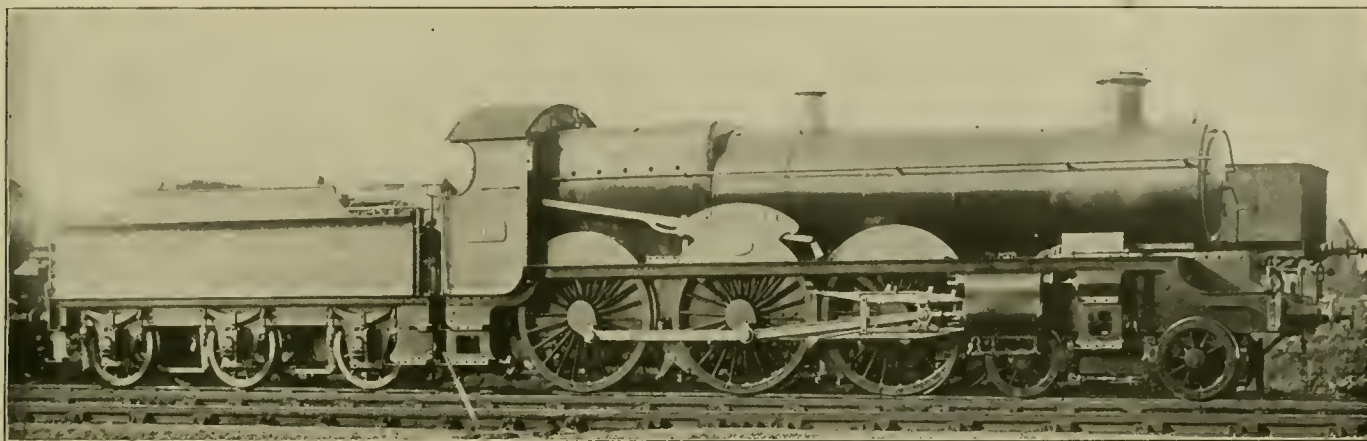
Great Western Six-Coupled, Four-Cylinder Superheater Locomotive
