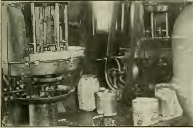
Equipment for Reclaiming Nuts
