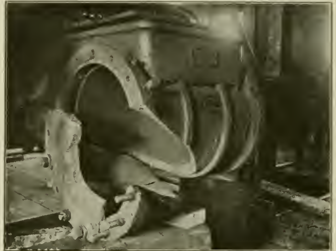
Fig. 1—Broken Locomotive Cylinder That Was Repaired by the Oxyweld Process
