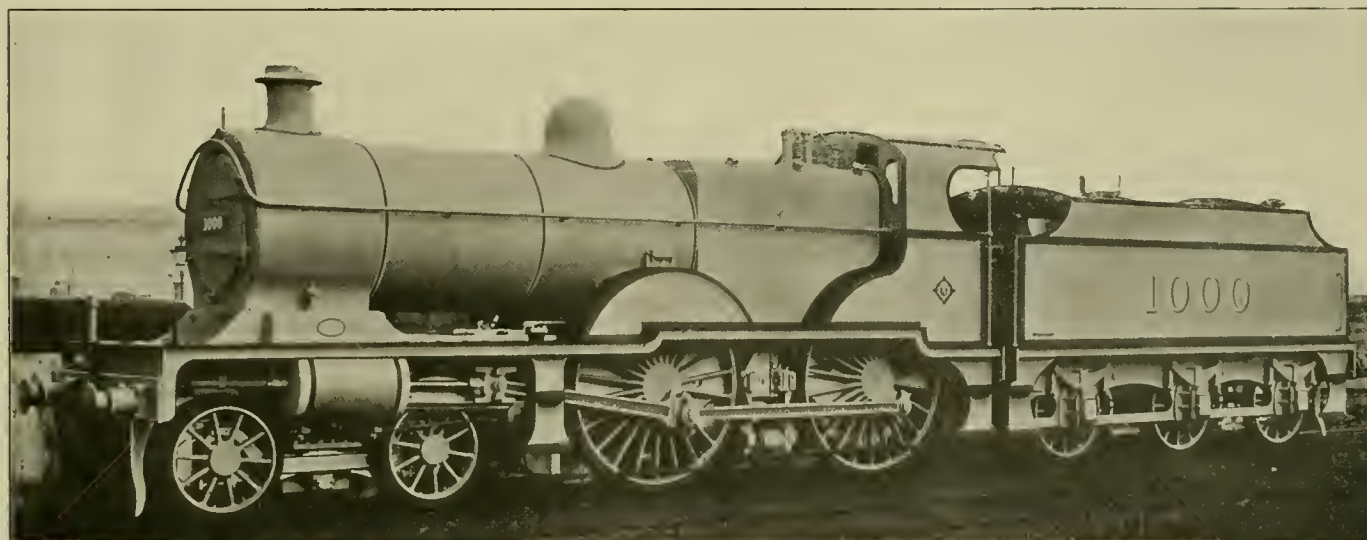
Four-Coupled, Three-Cylinder Compound Locomotive, Midland Railway
