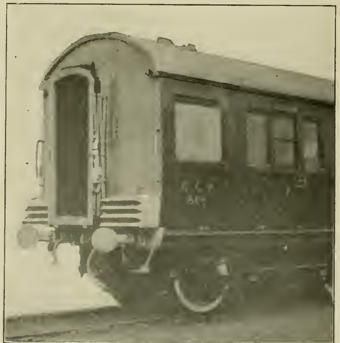
The Interlocking Fenders as They Appear on the End of a Car
