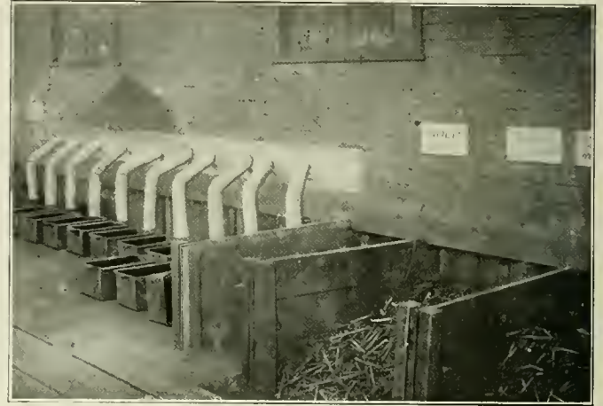
Delivery Chutes from the Nut Tapping Machines
