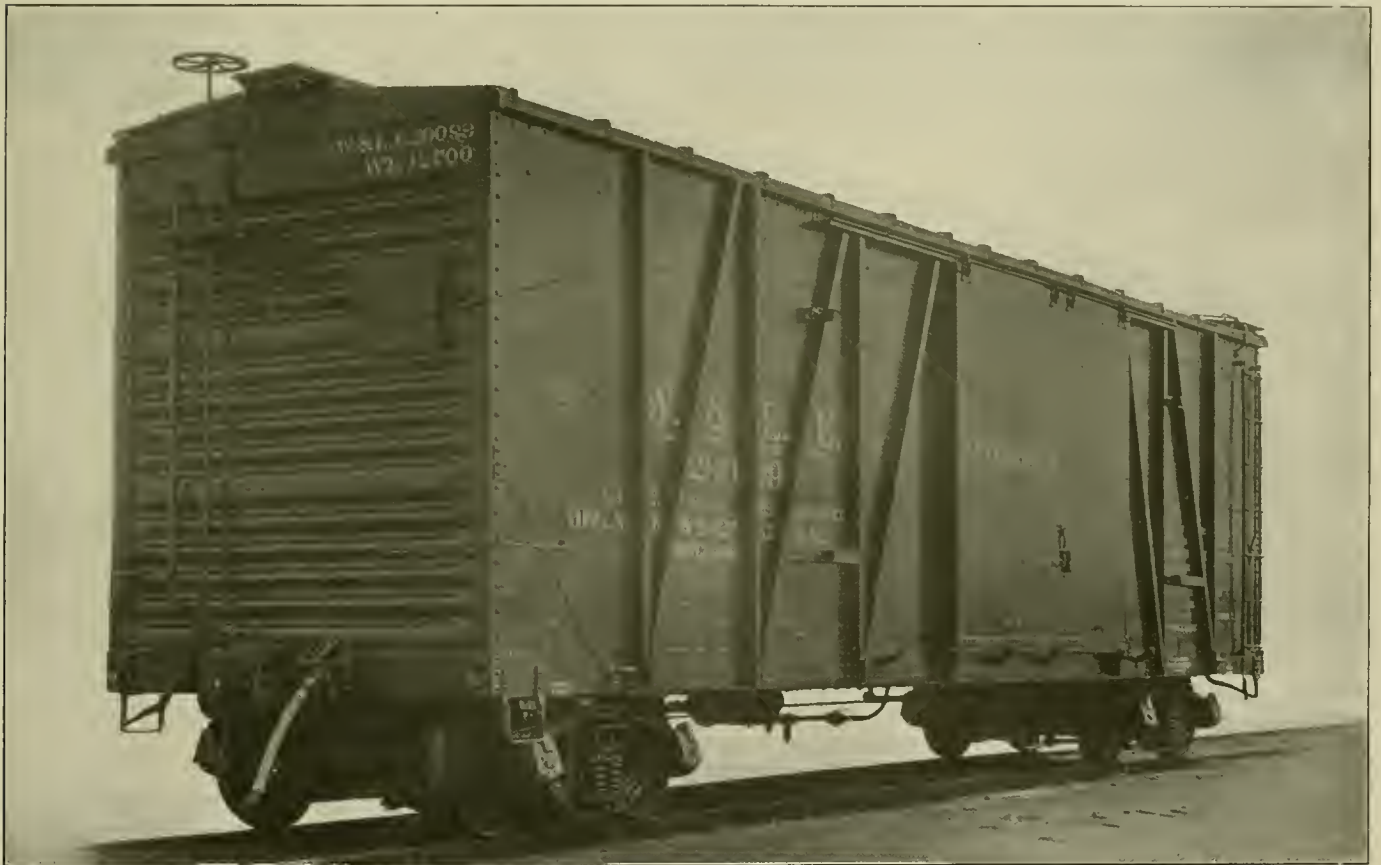
Wheeling & Lake Erie Steel Frame, Single Sheathed Automobile Car
