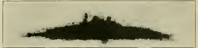
Record of the Movement of a Baggage Car Truck with Reference to the Car Body (slightly over full size)
