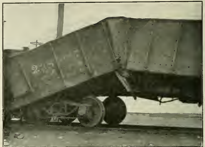
Fig. 4—A Steel Gondola Car Weakened by Corrosion and Buckled by Service Shocks
