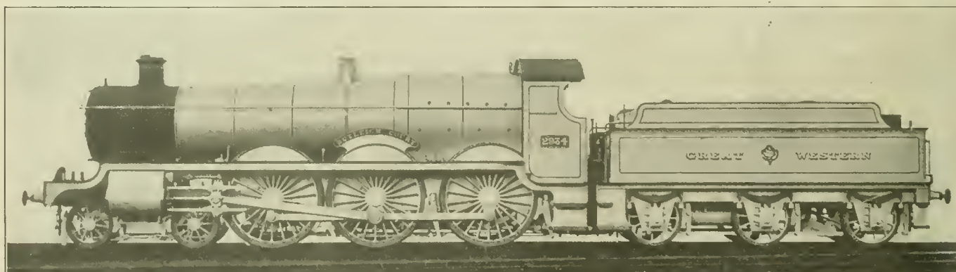
Great Western Six-Coupled, Two-Cylinder, Superheater Locomotive
