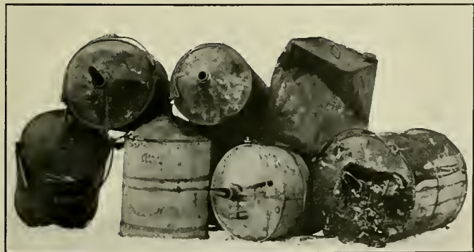
Poorly Designed Oil Cans Which Are Easily Injured and Require Considerable Storage Space
