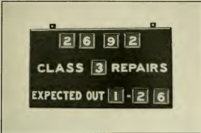
Locomotive Repair Indicator as Used in the North Springfield (Mo.) Shops of the Frisco
