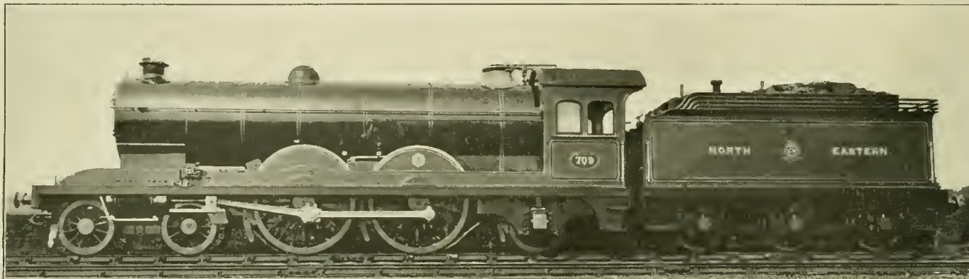
North Eastern Three-Cylinder, Atlantic Type Locomotive
