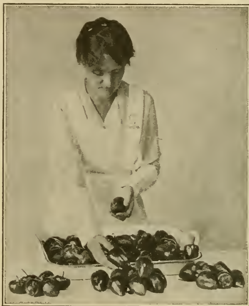
FIG. 1.—Sorting pimientos according to size and maturity before washing.
