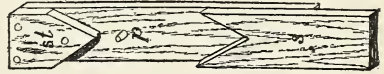
FIG. 76.—Cheshire anti-robbing entrance: st. , stationary piece; s. , slide; p. , pin or stop. (Redrawn.)
