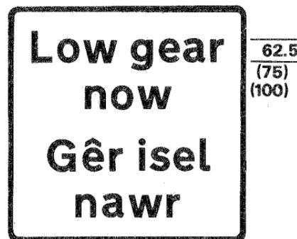
Plate for use with signs in diagrams 523.1 and 524.1
