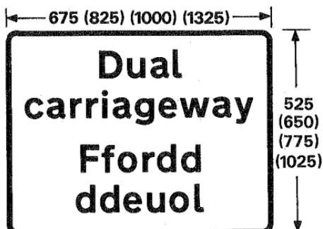
Plate for use with signs in diagrams 501, 601.1, 602, 606, 609 and 610
