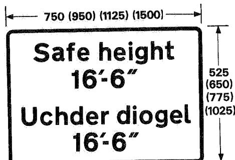
Plate for use with sign in diagram 533
