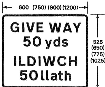
Plate for use with sign in diagram 501
