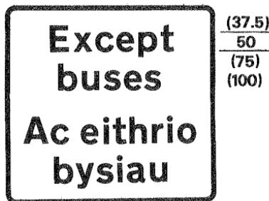
Plate for use with signs in diagrams 606, 609, 612, 613, 616, 619, 619.1, 626.1, 628.1, 629 and 629.2 and indicating exemption for stage carriages, scheduled express carriages, school buses and works buses
