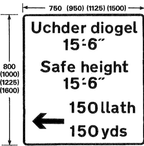
Plate for use with sign in diagram 533
