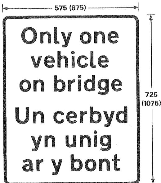
Plate for use with signs in diagrams 626.1 and 628.1
