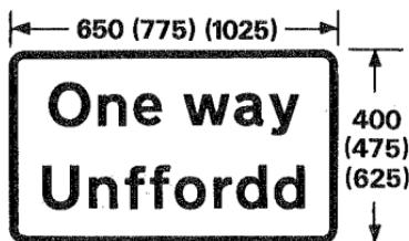
Plate for use with signs in diagrams 606 and 609
