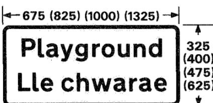
Plate for use with sign in diagram 545
