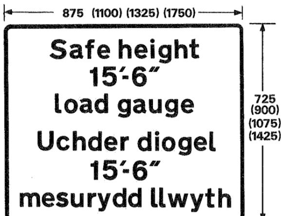
Plate for use with sign in diagram 533
