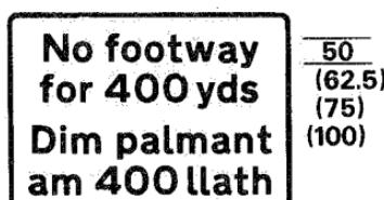
Plate for use with signs in diagrams 544.1 and 545
