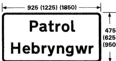
Plate for use with sign in diagram 545
