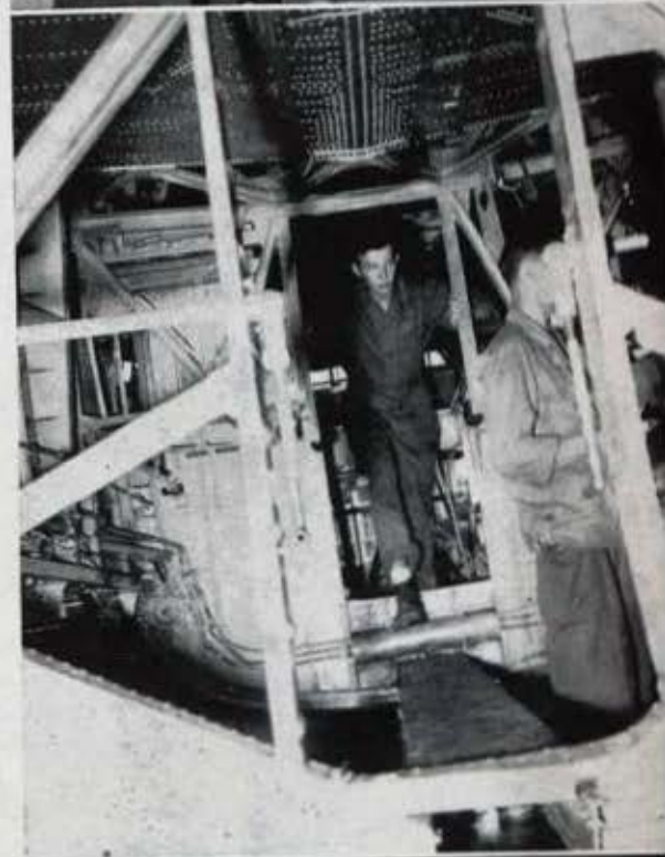
Examining nose gear shock strut.
