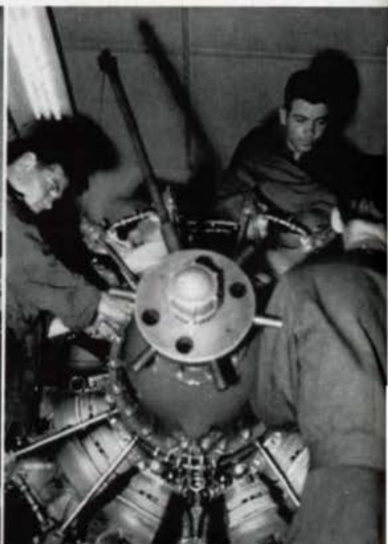
Installing aircraft cylinder.
