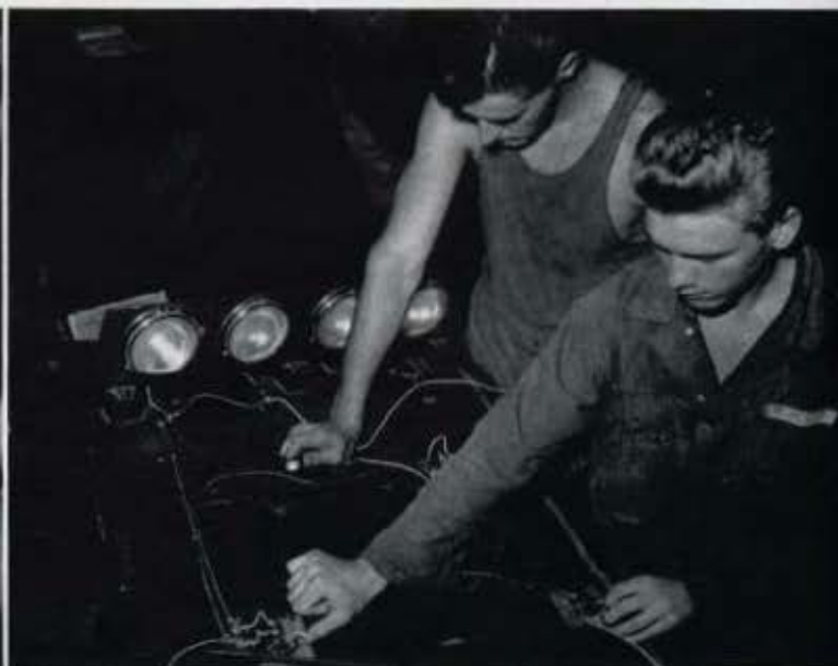
Bomb bay light circuit test.
