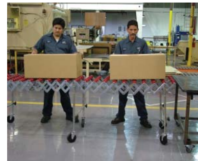
An expandable skate-wheel conveyor is portable and excellent where work needs to have a flexible layout.
