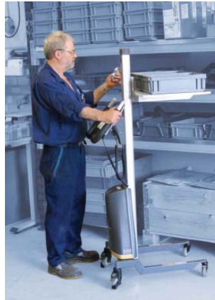
A manually propelled load lifter carries containers. The power lift raises and lowers containers to the appropriate work height.
