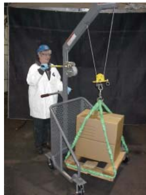
A portable hoist or “cherry picker” is manually operated. It is convenient for occasional spot-lifting of heavy loads.
