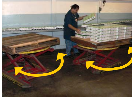
Turntable on a load leveler
