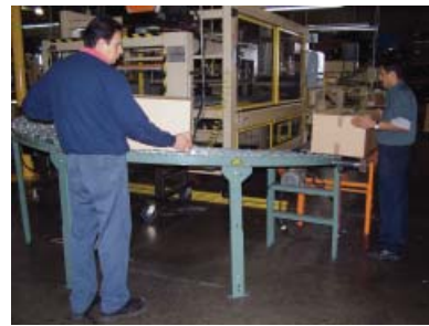
A curved skate-wheel conveyor moves containers around corners. It is activated by gravity.
