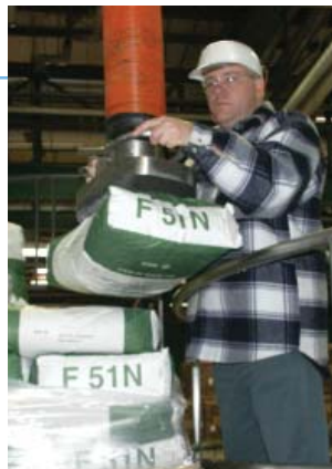
Vacuum lifters can handle sacks and bags that are hard to grip by hand.
