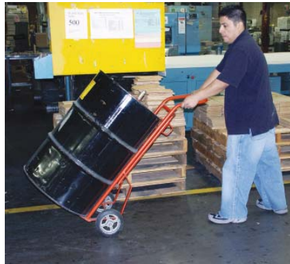
Two-wheel carts work well for loads up to about 300 pounds.
