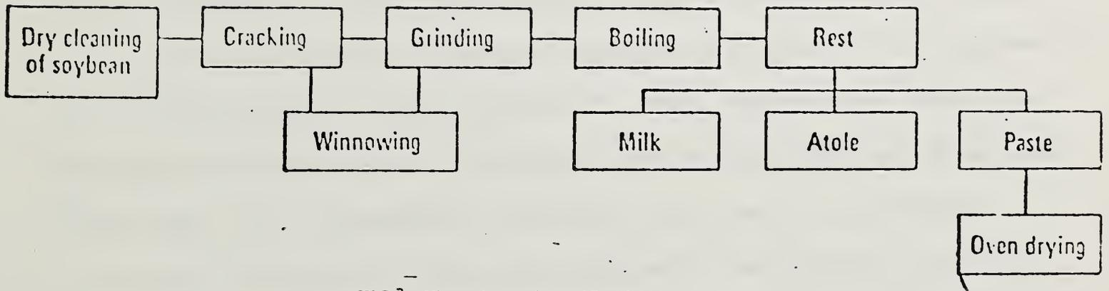
FIG.1. Flow chart of modified USDA process.
