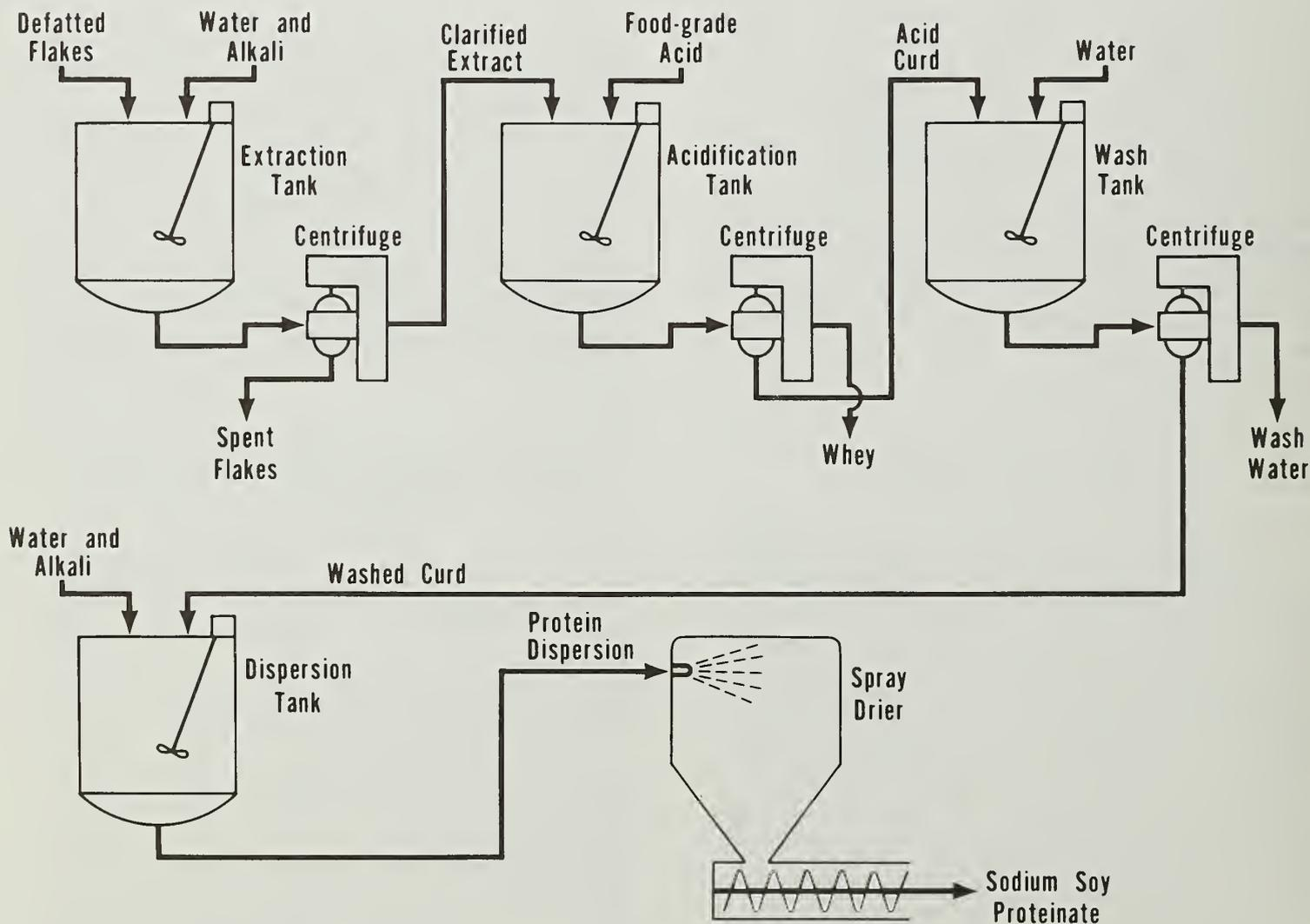
Figure 5.—Process for production of soybean protein isolates.
