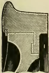
SECTION OF BOLTLESS FASTENING.
