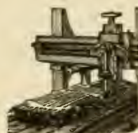
Radius Planer Attachment, for Planing Links on Planer.
