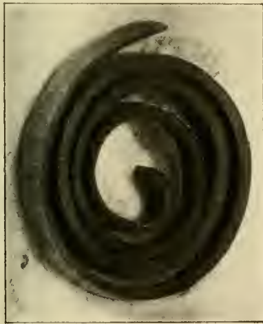
CHIP MADE WITH PNEUMATIC CHIPPING TOOL.
