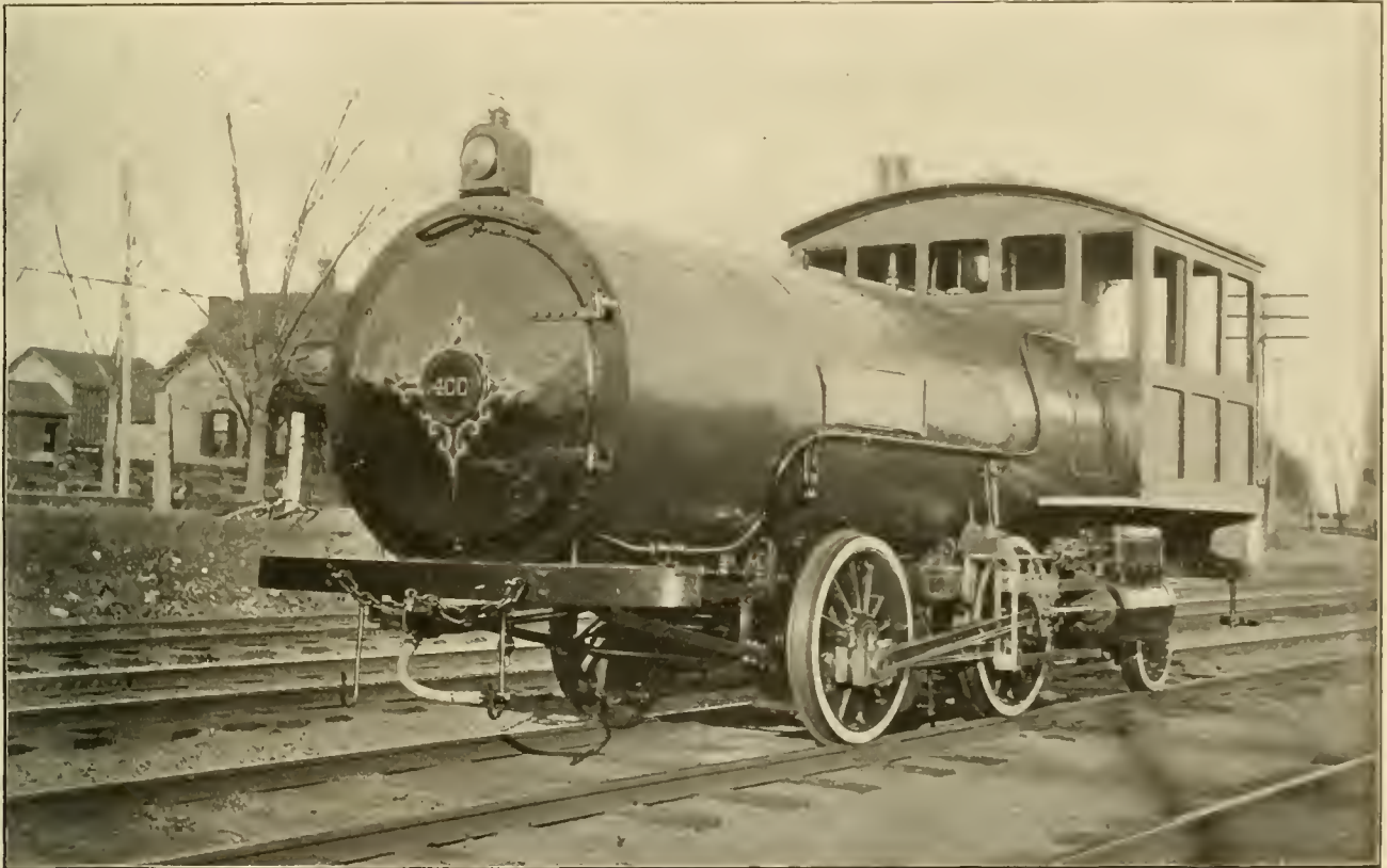
COMPRESSED AIR LOCOMOTIVE FOR NEW YORK ELEVATED RAILROAD.
