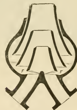
NEW SOUTH WALES EXHAUST PIPE.
