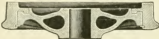
SECTION OF BOLTLESS FASTENING.
