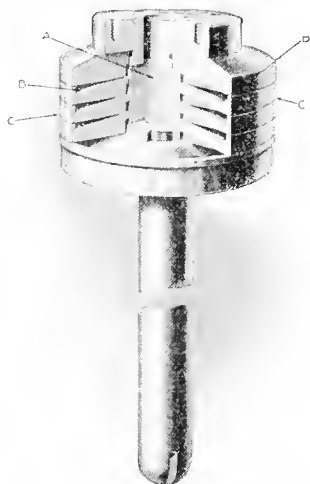
Fig. 91. The DeLaval emulsifier discs partially cut away to show the interior construction.
