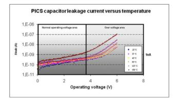
Figure 4: Leakage current vs. temperature
