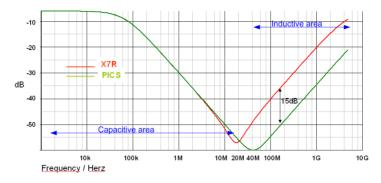
Figure 6: X7R and PICS capacitor insertion loss (100nF)
