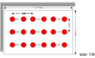
Figure 9: Current Ceramic Capacitor array
