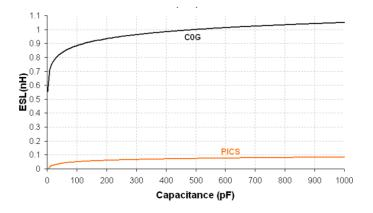
Figure 5: COG and PICS ESL versus capacitance
