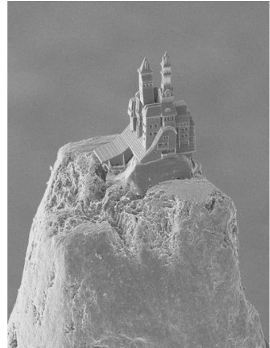
Castle 3D-printed on a pencil tip via multiphoton lithography. Author: Peter Gruber from Austria.
