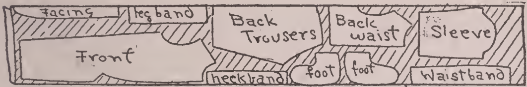
Fig. (170) A sample layout showing the pattern for the sleeping drawers placed on the goods
