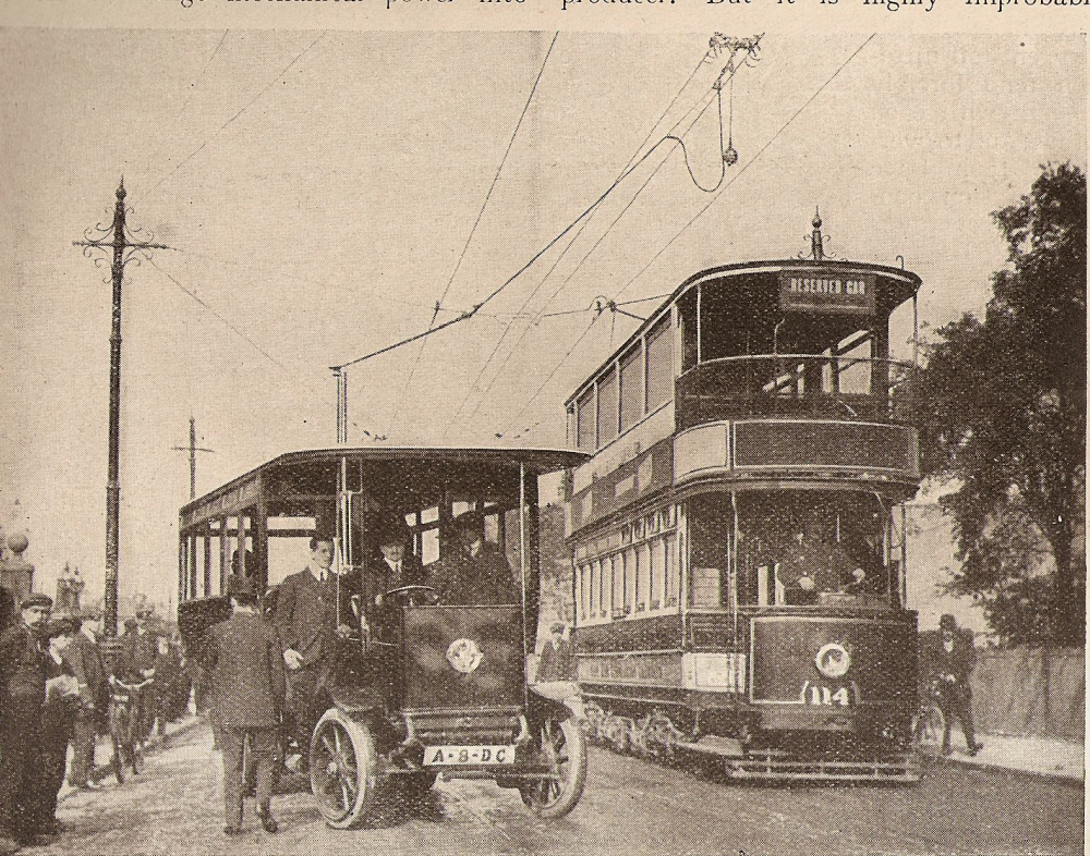
A NEW PHASE IN ELECTRIC TRACTION—THE TRAM ON RAILS PASSED BY THE TRACKLESS CAR
