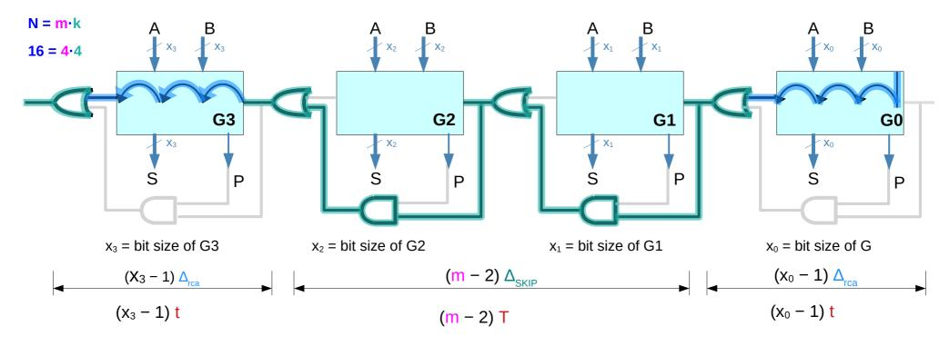
*t* denote the time required for a carry signal to ripple across a bit *T* denote the time required for the signal to skip over a group of bits *m* denotes the optimal number of groups for an n-bit carry chain
