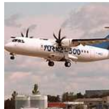
A smaller ATR-42, designed to carry 40-50 passengers.
