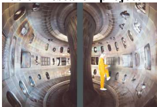
Scientist working inside a current fusion reactor; ITER will have 40 times the internal volume.
