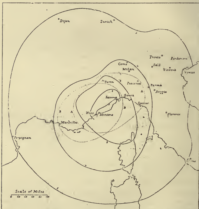
FIG. 33.—Isoseismal lines of the Riviera earthquake. (Mercalli.)
