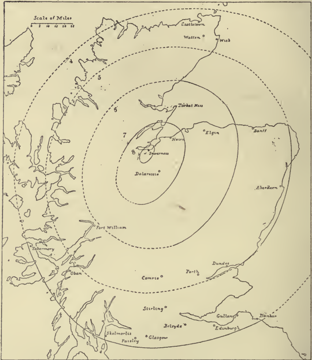
FIG. 65.—Iseismal lines of the Inverness earthquake. ( Davison. )
