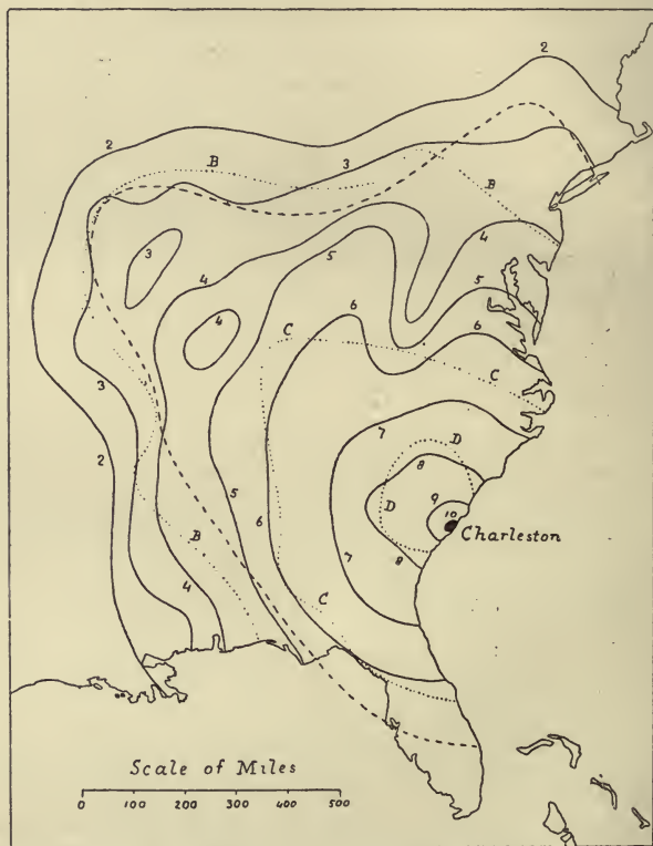
FIG. 25.—Isoseismal lines of Charleston earthquake. (Dutton, etc.)
