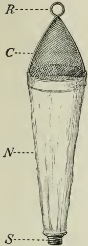
FIG. 3. — Birge's Cone Dredge. R. ring for attachment of line; C. wire cone; N. cloth net; S. screw cap.
