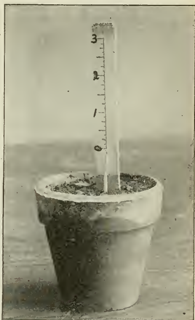
FIG. 4.—A more simple arrangement for measuring the growth of plants. Try it.
