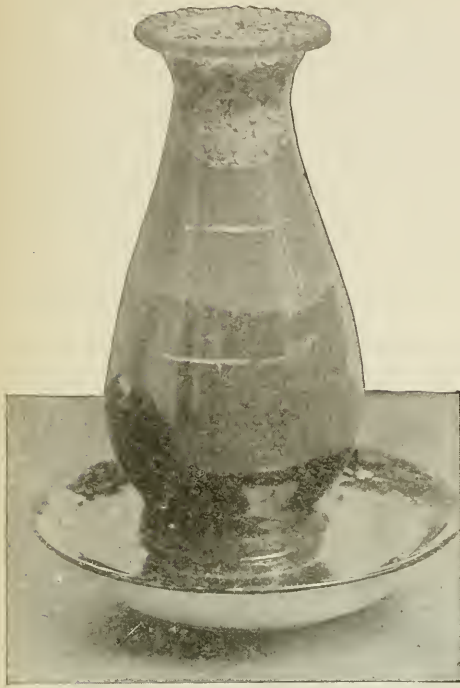
How water climbs through sand.
