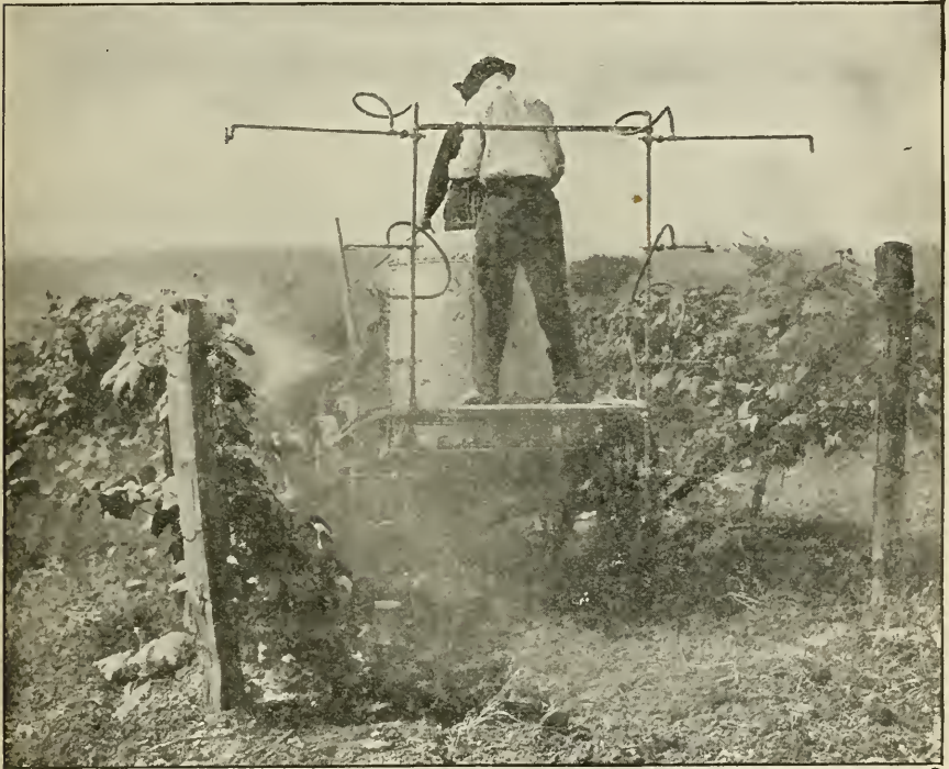
FIG. 43.—Carbonic-acid gas power sprayer at work in a vineyard. Spraying for the grape root-worm beetles.
