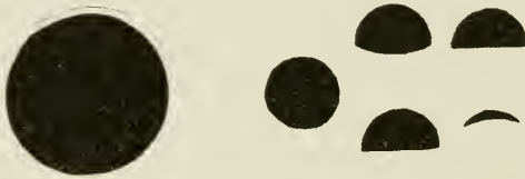
FIG. 170.—Diagram showing size of openings in various kinds of milk pails. The large circle at the left represents the common milk pail. The others show the perpendicular exposure in the new kinds of pails.
