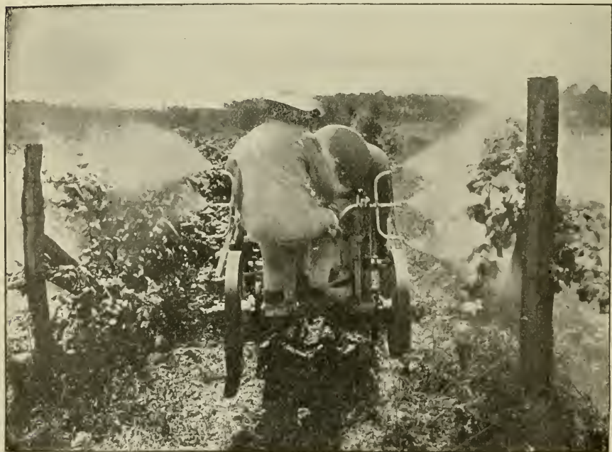
FIG. 45.—The vineyard sprayer shown in Fig. 44 in operation. The nozzles should be farther apart.
