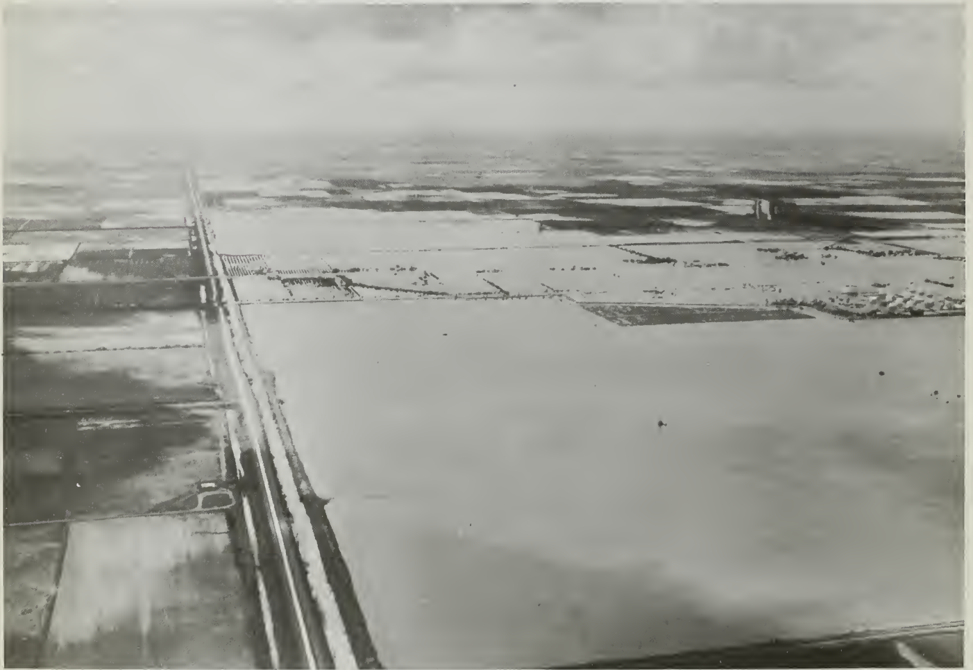
Removal of floodwater is delayed because movement is blocked by irrigation canal (thin white line), and because drainage ditch to the right of the canal is inadequate.
