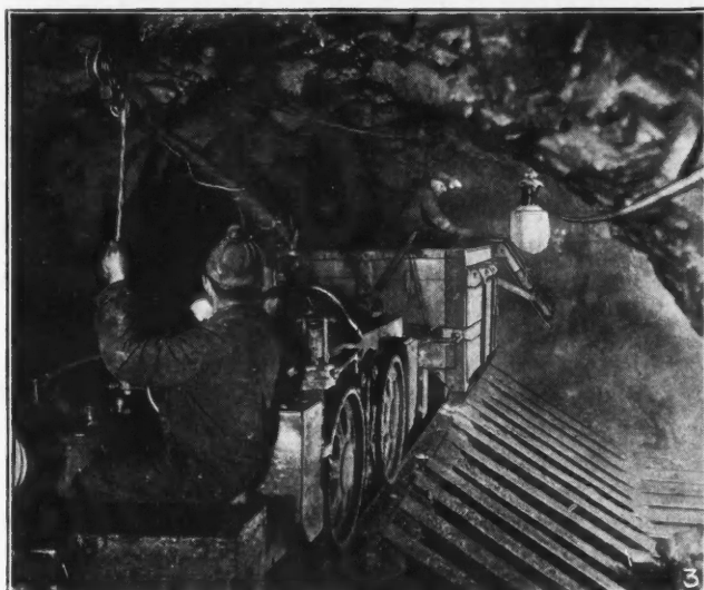
UNDERGROUND VIEWS AT REPLOGLÉ MINE. 1. MOTOR TRAIN ON FIRST LEVEL (STORAGE BATTERY LOCOMOTIVES ARE ALSO USED). 2. LOADING 4-TON MINE CAR AT STOPE CHUTE. 3. DUMPING INTO LOADING POCKET AT NO. 1 SHAFT. 4. BLACKSMITH SHOP AT FIRST LEVEL STATION
