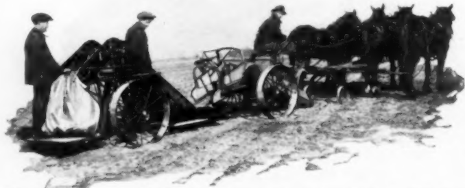
Digging Potatoes and Sacking Them in One Operation; the Outfit Will Harvest 600 to 800 Bushels in One Day
