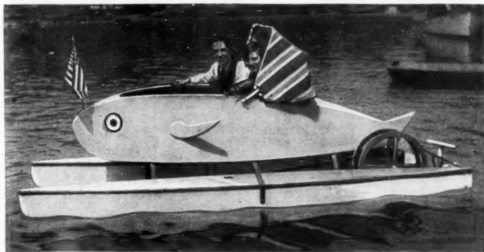
Like a Flying Boat without the Wings; Paddle-Wheel Craft, Operated by Hand, with Its Roomy Body and Folding Top; It Is Safe and Comfortable
