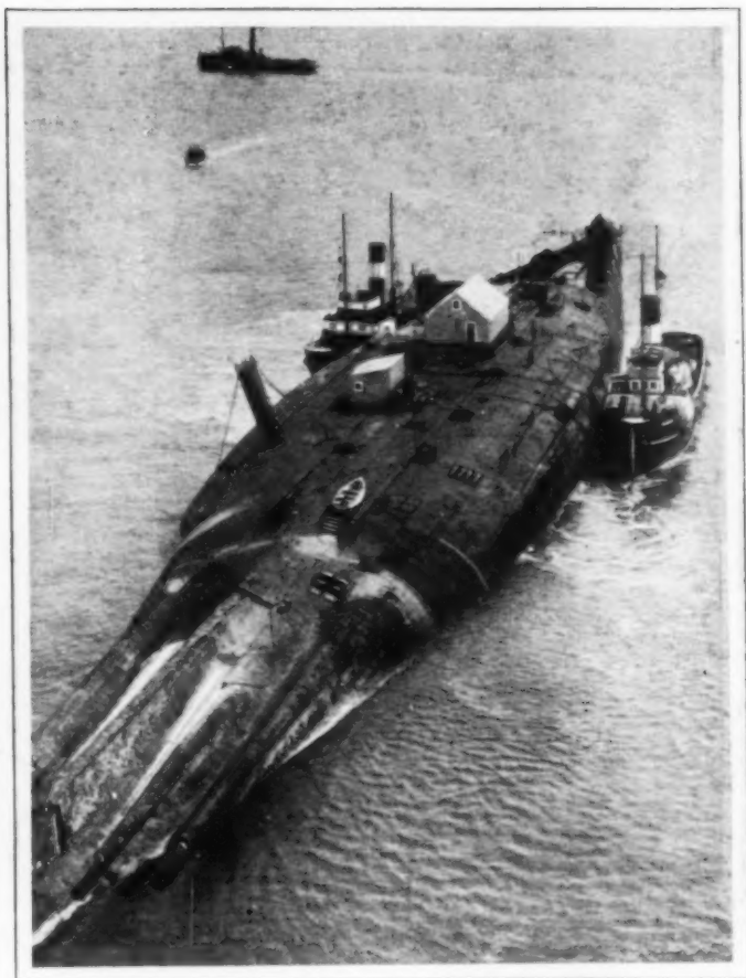
Bottom Up, the Cruiser "Moltke" Is Being Towed In for Dismantling and Salvaging as Steel Scrap
