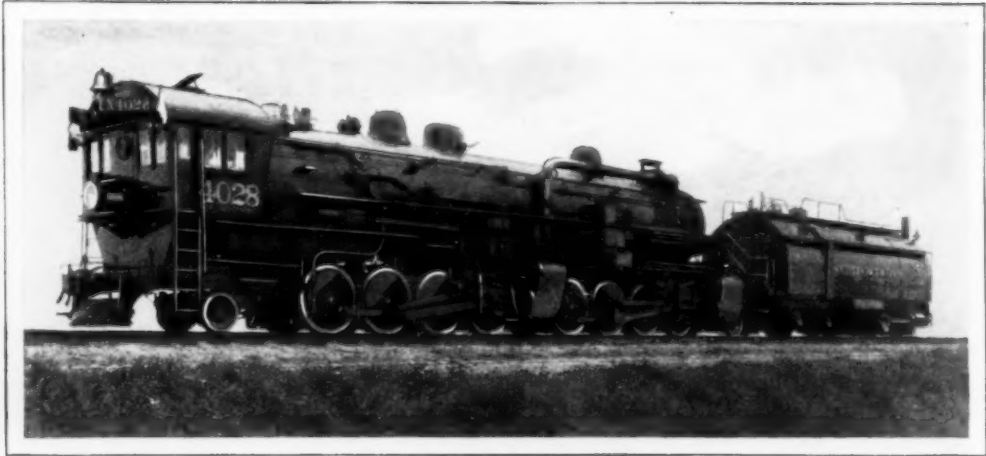
Remodeled Locomotive, with the Cab in Front for Easier Control of the Engine, Weighs 322 Tons and Is More Than 104 Feet Long
