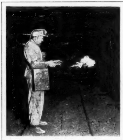
Studying Air Currents in Mine with the Aid of a Smoke Screen That Drifts with the Breeze
