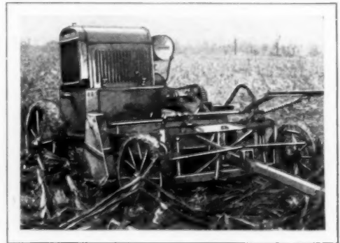
Motor-Driven Cutter That Chops Cornstalks into Small Pieces and Helps Check Spread of Insect Pest
