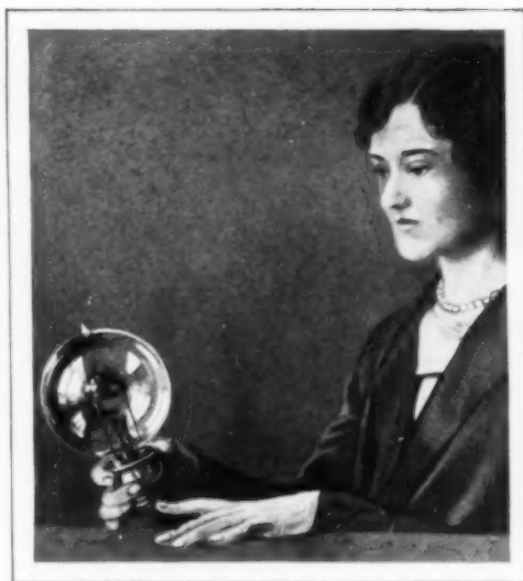
Midget Motor Used to Keep Time in Metering Operations at Electrical Laboratory
