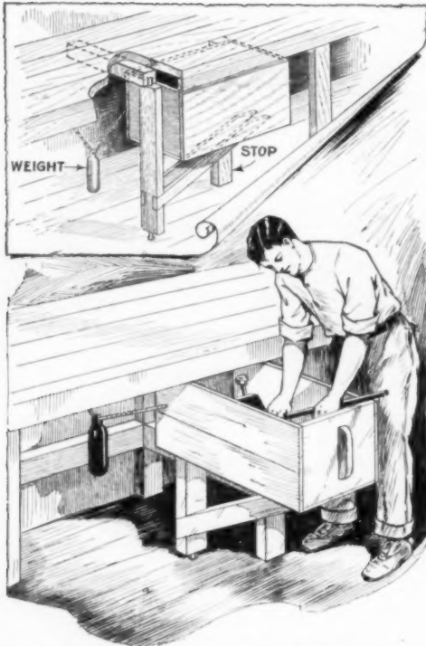
Workbench Drawer Which Can Be Opened and Closed Easily, No Matter How Heavily Loaded
