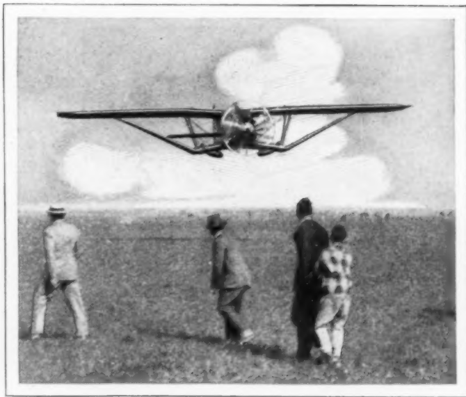
In Flight, with the Landing-Gear Wheels Folded Inward to Decrease Resistance from the Air, the Plane Develops More Speed
