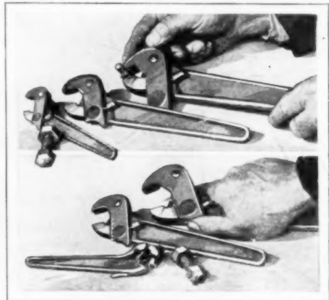
Three Wrenches Equal to Thirty; the Different Sizes and Method of Adjusting to Fit the Nut
