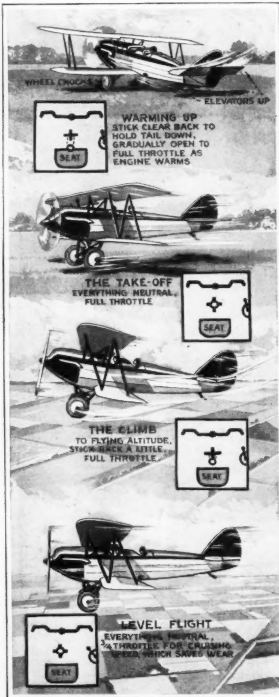
An Airplane Is Always Warmed Up on the Ground, to Bring It to the Best Operating Temperature; Then It Takes Off, Climbs for Altitude, and Levels Out
