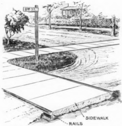
Road-Crossing Sidewalks Laid between Rails Are Fully Protected against Breakage
