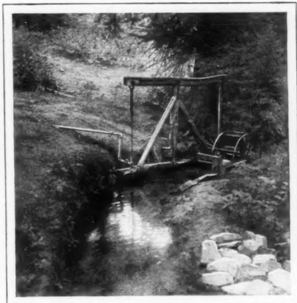
Small Waterwheel Installed in a Brook Operates a Pump Which Raises Water to a Near-By Reservoir
