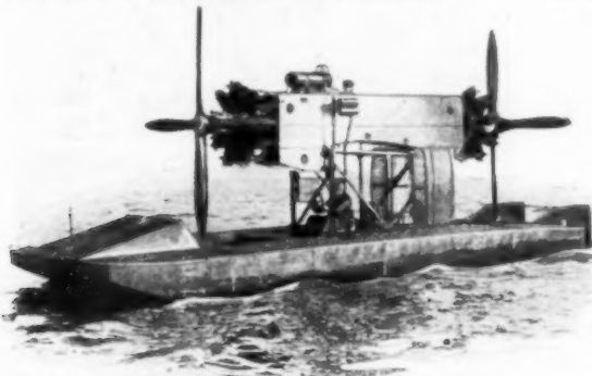
The Floating Testing Ground for Airplane Engines; Hydroplane with Motors Installed for Trial Run
