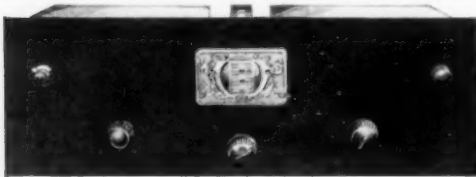
Front Panel Showing, from Left to Right, Switch and Trimmer Condenser Knobs, Dial Knob, and Rheostat and Tickler Knobs
