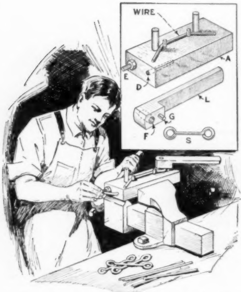
A Simple Jig Which Will Facilitate the Making of Links of Equal Size
