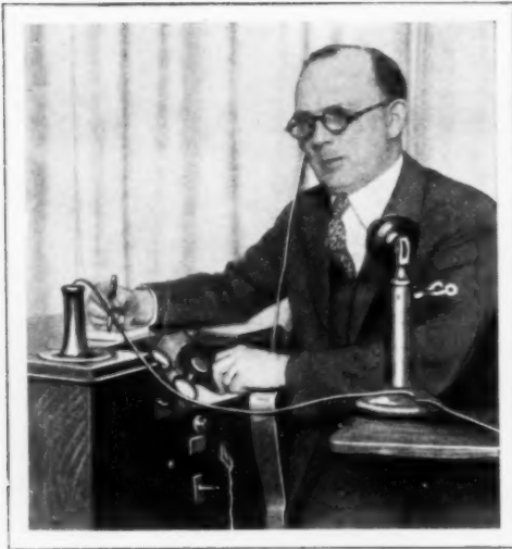
Telephone Conversation Being Amplified through the Cabinet That Aids the Hard of Hearing
