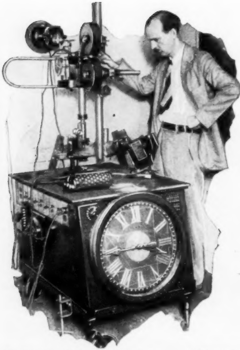
Combination Motion-Picture Camera and Microscope Operated by Clockwork for Filming Germ Life
