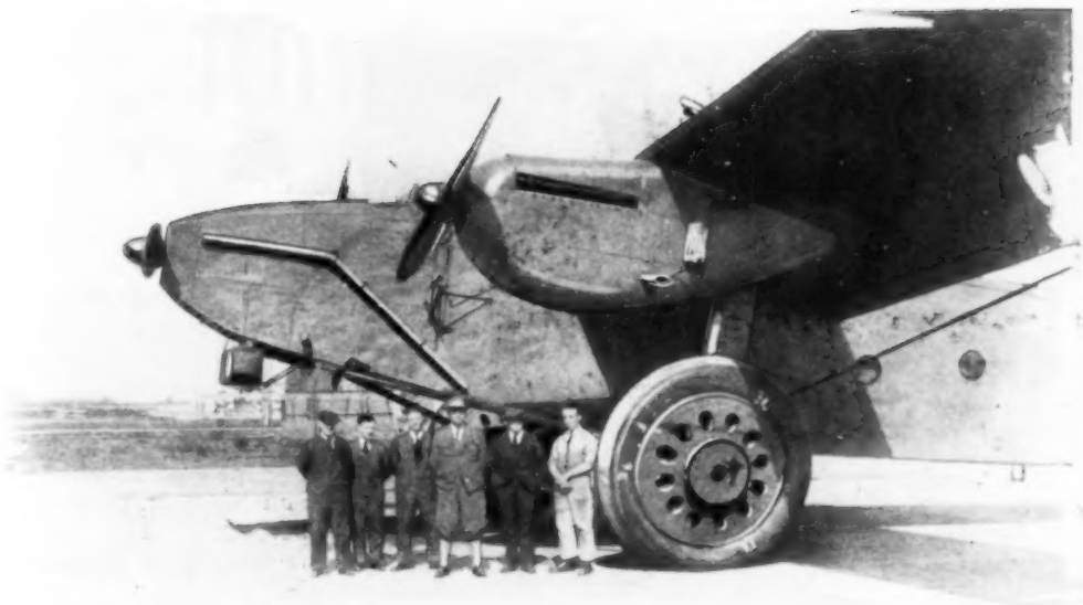
Giant Tires Were Required When England's Newest Bomber, the Beardmore "Inflexible," Took the Air; the Huge Tri-Motored Monoplane Is the World's Biggest Ship of Her Type
