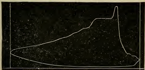
Diagram from 18" x 36" engine with cut-off valve operated by Kendal Governor.
