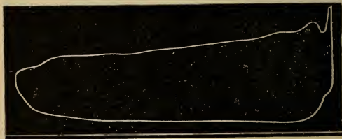
Diagram from same, 9' x 15' engine, with different valve setting.
