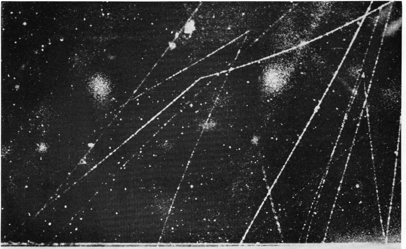
Three of the baffling V particles whose existence was recently confirmed here at Tech. They are formed by cosmic rays hitting the nuclei of lead atoms.
