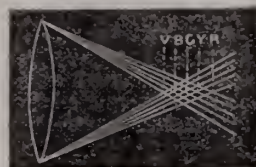
Chromatic dispersion by a single lens.
