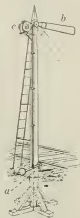
Railway Semaphore. a, lever, which operates both b, blade, and c, lantern.
