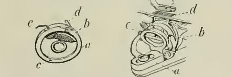
shaft of small driving-wheel *c*, which is driven by the belt *d* from the main driving-wheel; *e*, stitch-regulator, which,
