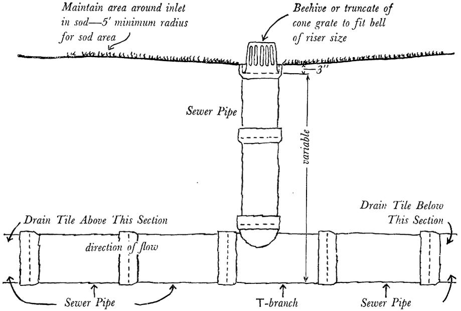
A small surface inlet made of sewer pipe for use on lateral tile lines. (See pages 508-520.)
