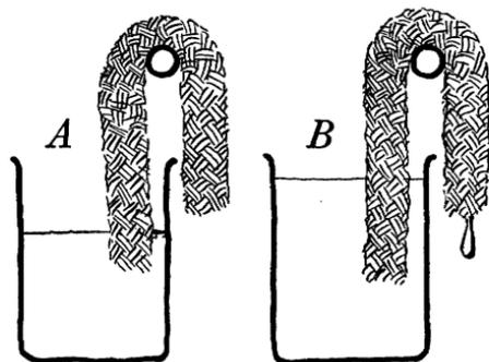
*Surface tension action in a wick illustrates hydrostatic balance and viscous flow in soil.*
