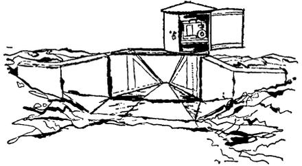
*Weir and water stage recorder for measuring runoff.*
