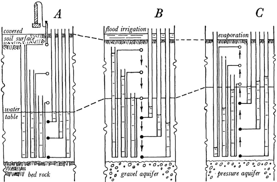
Hydraulic-head relations in three soil profiles, representing A, hydrostatic balance; B, downward flow; C, upward flow.
