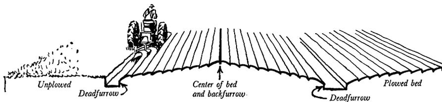
*Cross Section of Bed Showing Construction Method*
