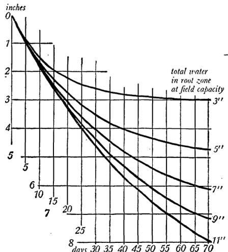
This sketch shows actual rate of soil moisture depletion from soils holding different amounts of water in the root zone, assuming a constant rate of potential evapotranspiration of .2 inch a day.
