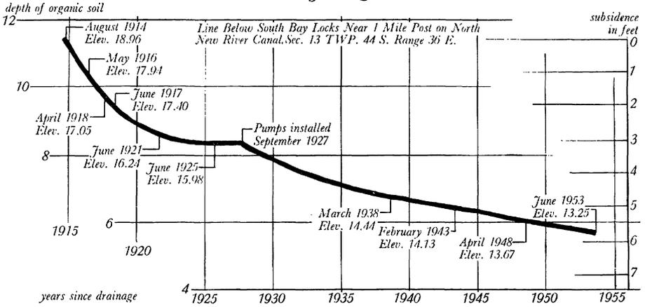
The subsidence rate of a drained organic soil over a period of nearly 40 years. The normal pattern of fast sinking of the surface with initial drainage, a leveling off as gravity drainage decreased, an increase in rate with better drainage due to pumping, and the steady loss of surface elevation thereafter are illustrated. Soil is Okeelanta peaty muck near South Bay, Florida. (See pages 539-557.)
