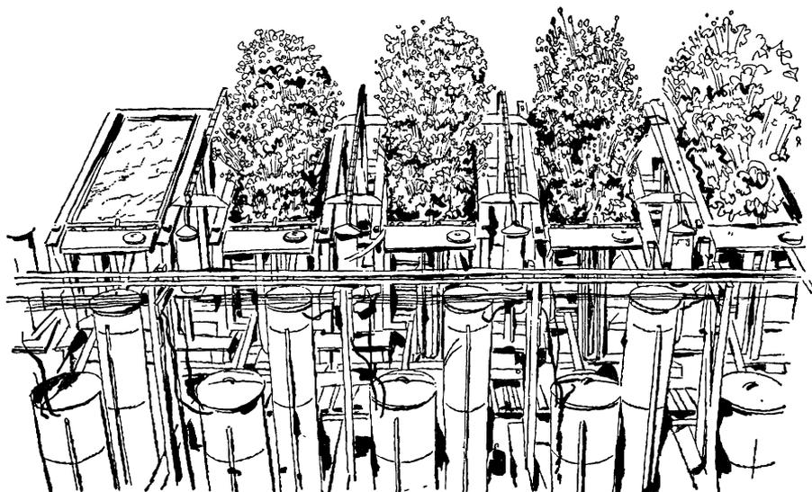
*A battery of small lysimeters, instruments that measure the effect of plant cover on the movement of water over, in, and through the soil.*
