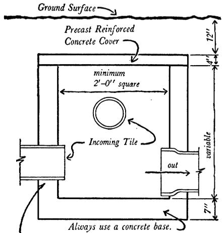
Construct walls of concrete, brick, block or curved segment
