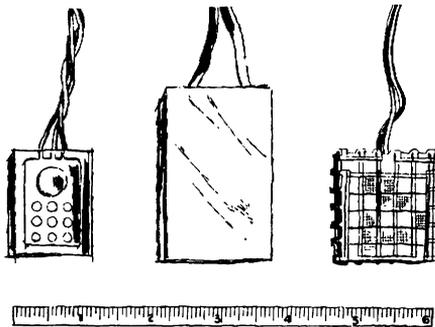
Resistance units for measurement of soil moisture. (Left, fiberglass; center, plaster of paris; right, nylon.)
