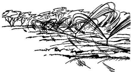
*Double-nozzle, revolving-head sprinklers spaced 40 feet apart on a portable "quick-coupled" aluminum lateral line.*
