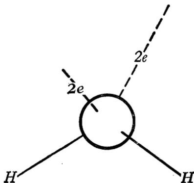
In the diagram above of the water molecule, the dotted lines symbolize the hydrogen-bonding tendency arising from the diffuse cloud of electrons in the direction of the dotted lines. Several molecules held together by hydrogen bond, as in solid or liquid water, form an assembly of tetrahedral groups; each molecule is bonded to four other molecules, which it closely approaches.
