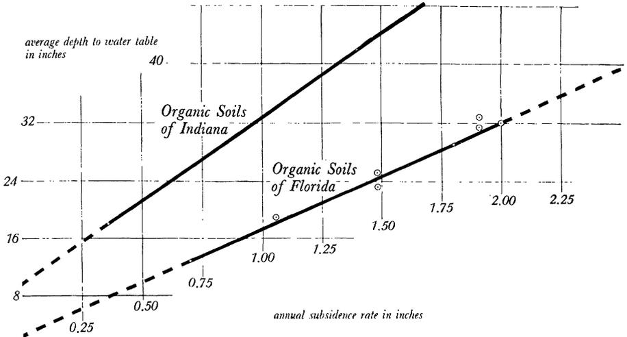
This shows that the subsidence rate for organic soils depends on the depth to the water table. The lower the water table, the greater the soil loss. Data from Indiana based on drainage depth during crop year, May to September only. For Florida, drainage depth was held the whole year. (See pages 539-557.)
