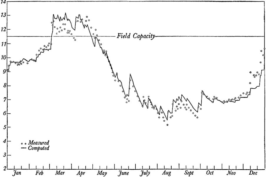
Soil moisture in 0-40' profile on Watershed T102, Coshocton, Ohio, 1944. Measured values obtained by Soil Conservation Service from soil samples and by use of weighing lysimeter. Computed values are from daily climatological data; the water budget method was used.
