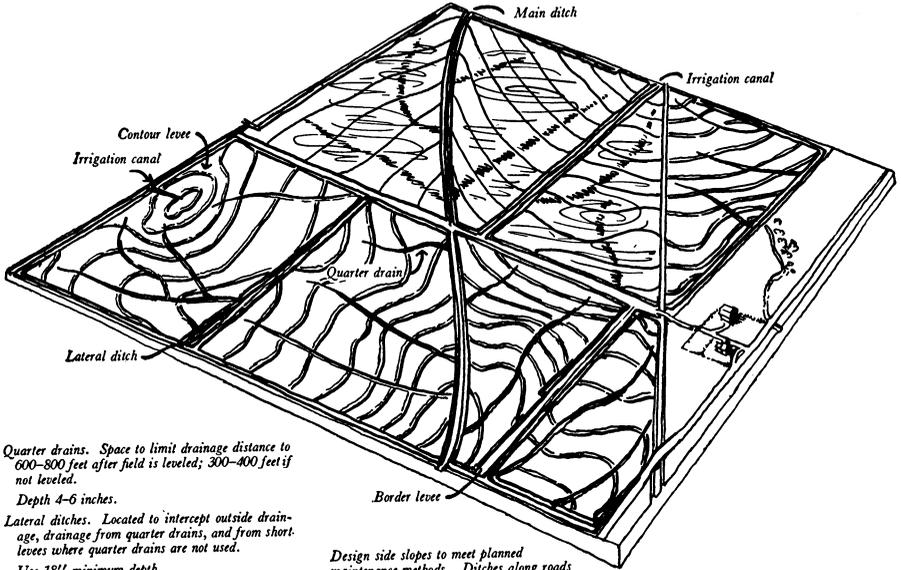
Quarter drains. Space to limit drainage distance to 600-800 feet after field is leveled; 300-400 feet if not leveled.
