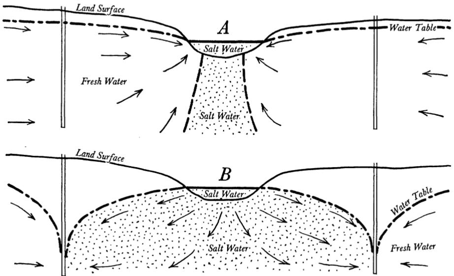
FIGURE 1. This diagram shows the ground-water conditions near a tidal stream that usually carries salty water in its channel. The arrows indicate the direction of ground-water flow. Salt water underlies the stream channel as a trapezoidal prism. A is the movement under natural conditions before pumping takes place. B is the movement during pumping of ground water. A cone of depression surrounds each pumped well, the water table is depressed, and salty water encroaches into the aquifer.
