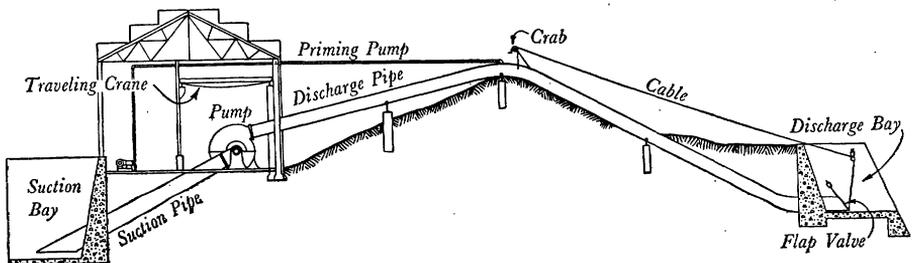
*Elevation of well-designed pumping plant; reinforced suction and discharge bays (piling not shown; inclined suction pipe; discharge pipe over top of levee with long radius bends; crab for lifting flap gate. (See pages 528-538.)*
