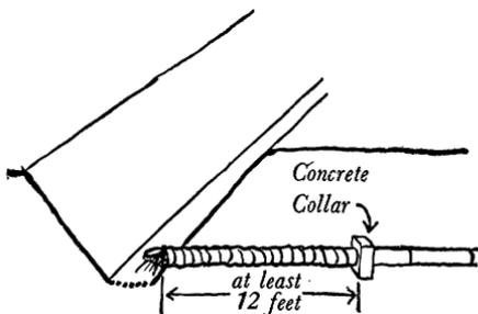
*When no surface water will enter the ditch at the location of the tile outlet, a section of continuous rigid pipe gives the best outlet protection.*
