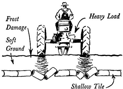
Shallow tile may be damaged by frost and heavy modern machinery.
