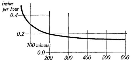
*Infiltration under average soil moisture and temperature during 149 storms—row crop, C soil group. (A list of soil groups is given on page 157.)*
