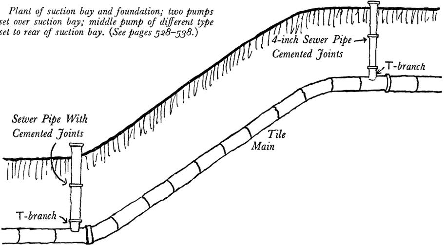
A drawing showing the placement of a breather near the beginning of a steep grade and a relief well at the end. (See pages 508-520.)
