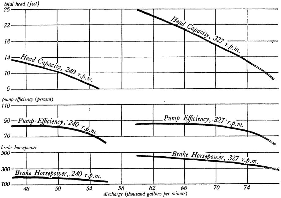
Characteristic curves of mixed-flow pump; field tests 48-inch pump; Green County, Ill.
