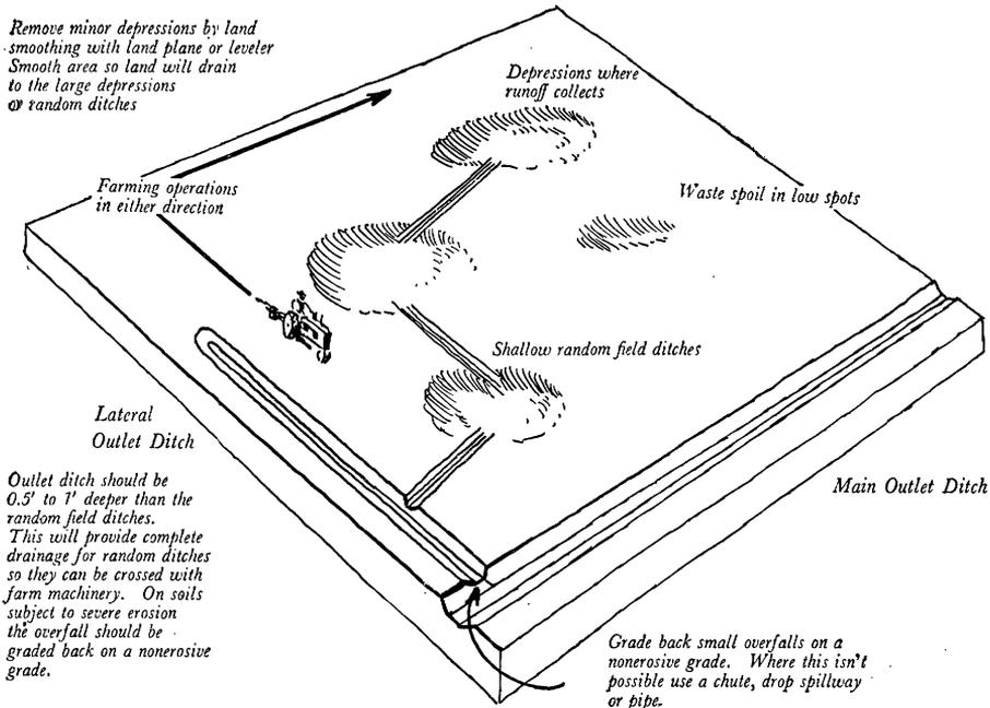
Outlet ditch should be 0.5' to 1' deeper than the random field ditches. This will provide complete drainage for random ditches so they can be crossed with farm machinery. On soils subject to severe erosion the overfall should be graded back on a nonerosive grade.
