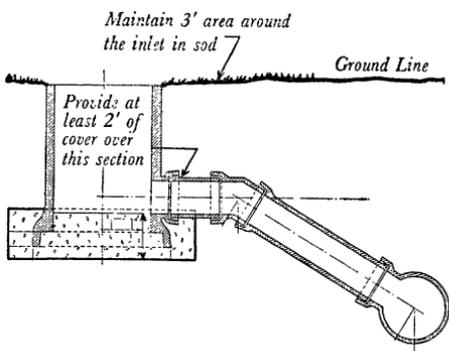
*Open surface inlet located off to one side of tile main. A larger sewer pipe T-branch is used for the riser.*
