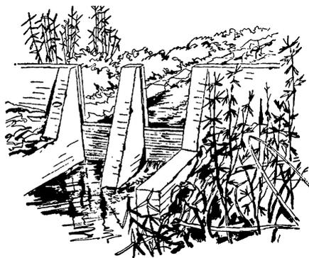
The flashboard type of structure is probably best adapted to this need. Its design should provide for an ample spillway space above the flashboards when they are in place at their highest level. They have been built with reinforced concrete; concrete precast blocks, using steel reinforcing bars and concrete filling of the voids in the block; and braced steel H-columns. All are satisfactory if properly built.
