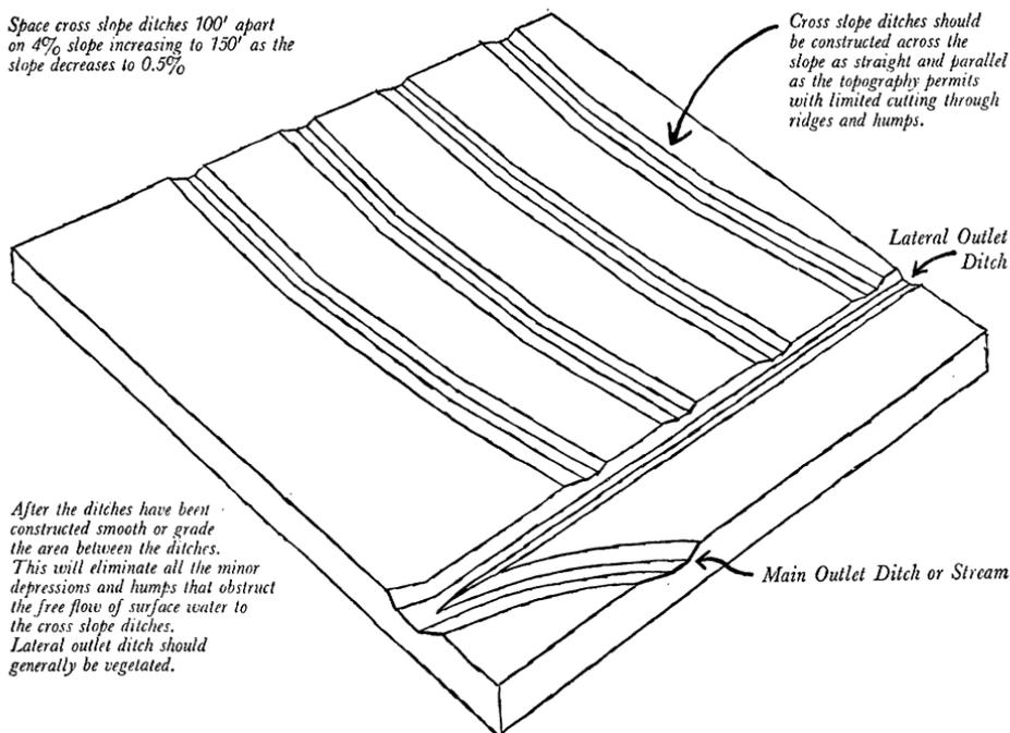
After the ditches have been constructed smooth or grade the area between the ditches. This will eliminate all the minor depressions and humps that obstruct the free flow of surface water to the cross slope ditches. Lateral outlet ditch should generally be vegetated.
