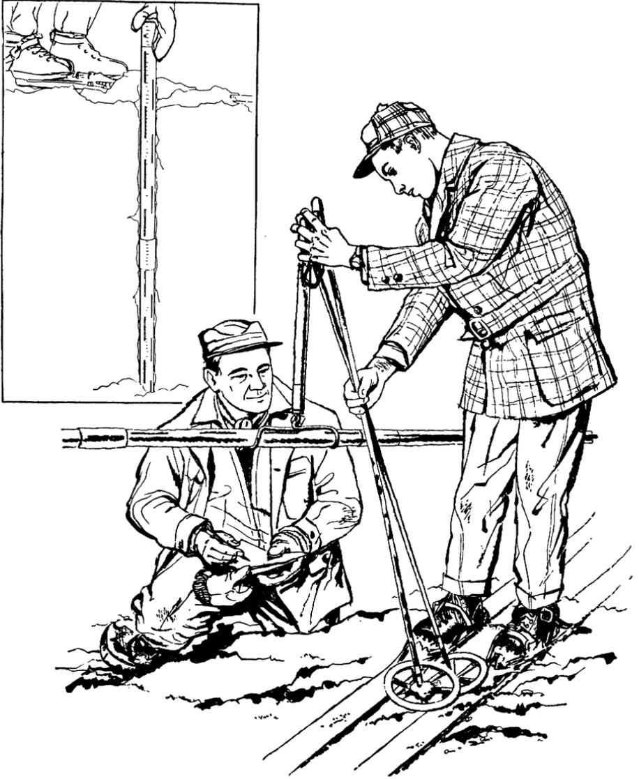
*Measurements of deep snow are made by coupling together sections of the lightweight tubing, calibrated into  $\frac{1}{2}$ -inch divisions along its entire outer length. Thus the depth of snow can be read after the sampler has been driven to the soil beneath.*
