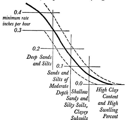
The range of minimum infiltration rates with row crops on wet soils. The variation due to past treatment is shown by the dashed line about the mean.
