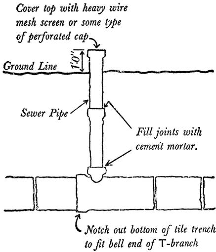
Breather or air vent. Can be used as a relief well by increasing size of the riser pipe. (See pages 503-520.)
