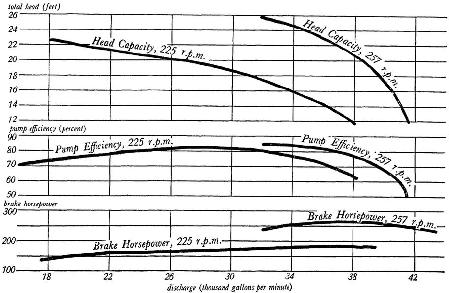
Characteristic curves of centrifugal pump; field tests of 36-inch pump; Adams County, Ill. (See pages 528-538.)
