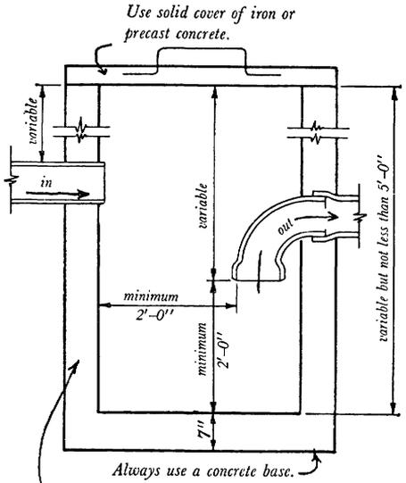
Construct walls of concrete, brick, block, curved segment, concrete or sewer tile.
