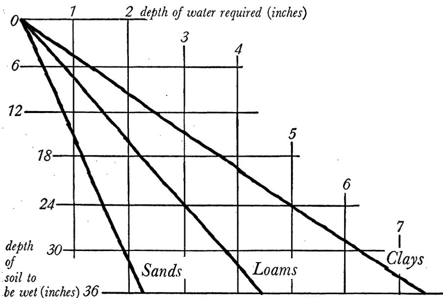
Surface inches of water required to wet dry soils to given depths assuming no surface runoff. How to read the chart: Assume a 12-inch depth of loam soil is to be wet. Run down left-hand scale to 12-inch line, then across chart to intersection with diagonal line labeled "loams," and then project line vertically up to scale across top of chart. Depth of water required is 1.5 inches.
