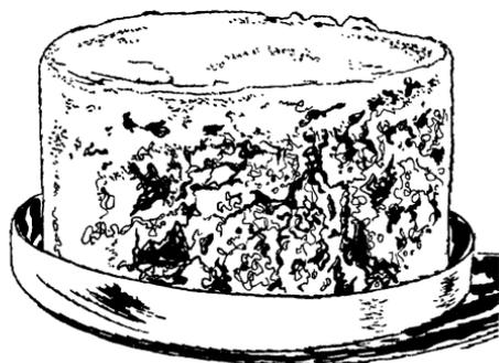
*Surface seal on a core sample of freshly plowed cropland after a 20-minute test application of water drops by a raindrop applicator.*
