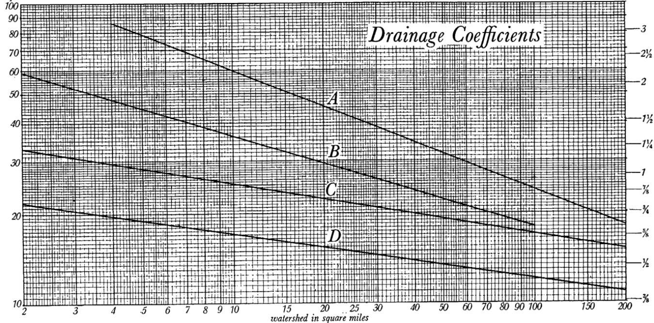
A—For good protection from overflow (not maximum flood runoff). B—For excellent drainage. C—For very good agricultural drainage in Ohio, Indiana, Illinois, Iowa, and northern Missouri. D—For fair agricultural drainage in Ohio, Indiana, Illinois, Iowa, and northern Missouri. Watershed area to be determined above each section of a ditch for which capacity is to be computed. Applicable only to flat watershed areas having average slope less than 25 feet per mile.
