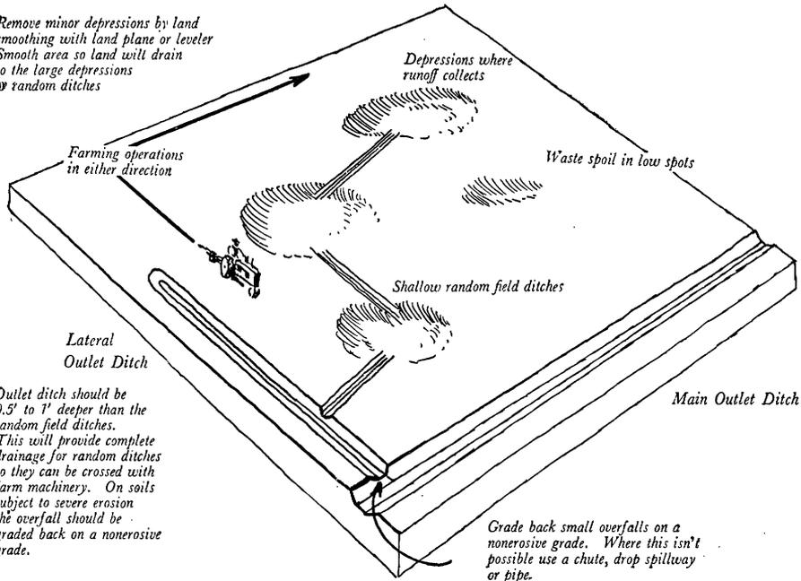
Outlet ditch should be 0.5' to 1' deeper than the random field ditches. This will provide complete drainage for random ditches so they can be crossed with farm machinery. On soils subject to severe erosion the overfall should be graded back on a nonerosive grade.
