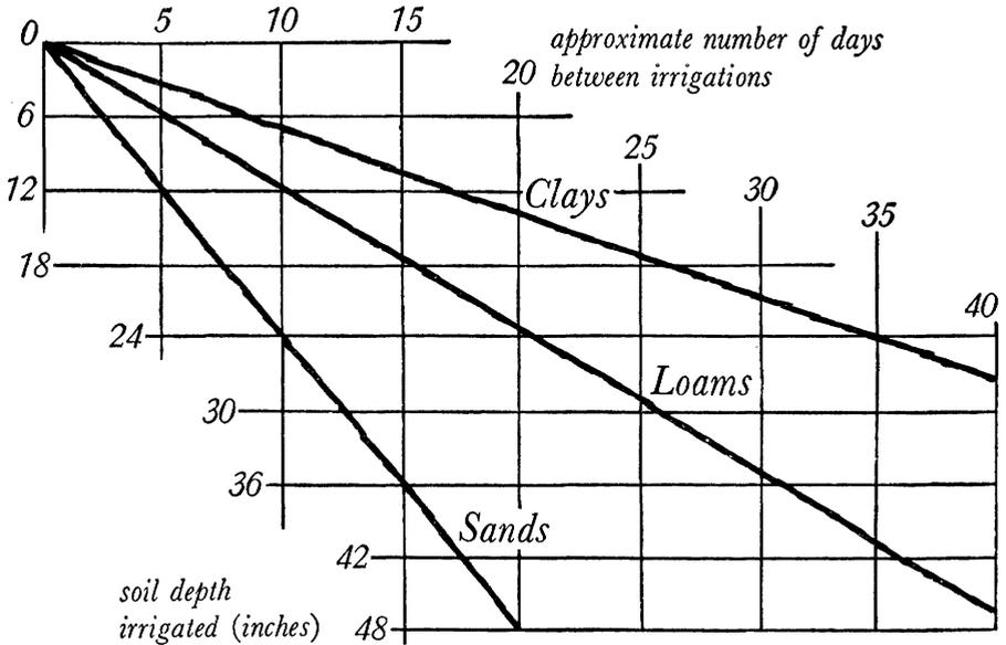
*Irrigation interval as influenced by soil texture and depth of root zone wet where water use is 1 inch a week. How to read the chart: Assume grass has effective roots to 24-inch depth and soil is wet to this depth. Run down left-hand scale to 24-inch line, then across chart to intersection with diagonal line labeled "loams"; and then project line vertically up to scale across top of chart, where you read off about 21 days.*
