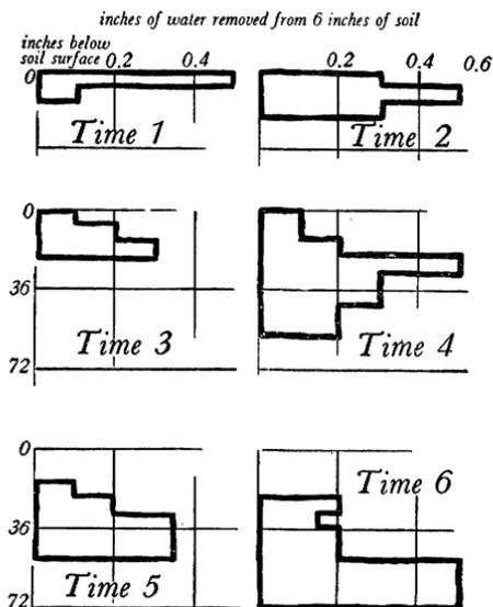
Water removal patterns for Millville loam for successive time intervals after a thorough irrigation. Water is first removed from the surface soil; as the moisture is reduced, it becomes harder to get and removal comes from successively lower depths. The total water removed in any time interval depends on weather and stage of growth of the plant.
