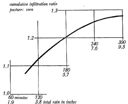
The relative infiltration of bluegrass pasture to corn on silt loams of C Group. The relative increase on deep silts may be greater than that shown; the relative increase on sands may be less. Lateritic soils may also be less than that shown by the curve, although greater than for sands.
