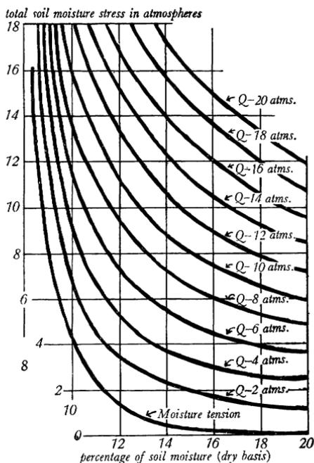
The relationship between total soil moisture stress and moisture content of a Panoche loam with various increments in osmotic pressure of the soil solution induced by added salt.
