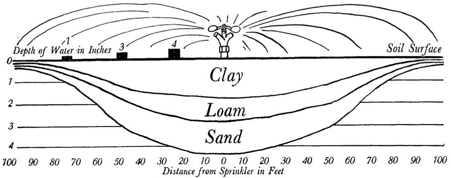
*Distribution of water under a single rotary sprinkler. Depths of water collected in cans placed along surface show progressively less water is applied with increasing distance from sprinkler head. This is reflected in depth of soil wet. To obtain uniform application, sprinklers must be lapped. The depth of soil wet by a given application of water is determined by its texture (sand, loam, or clay).*
