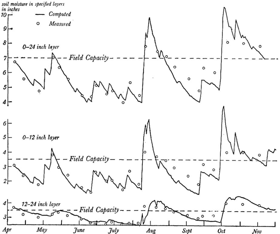
Soil moisture in specified layers of soil profile, College Park, Md., 1942. Measured values obtained by Soil Conservation Service from soil samples. The values were computed from daily climatological data, the water budget method was used.
