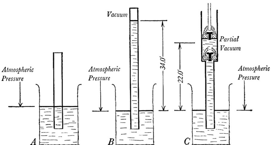
*Suction lift caused by atmospheric pressure. A, No lift or rise inside tube when pressure inside and outside are equal; B, suction lift, with complete vacuum inside tube (theoretical); C, suction lift of pump with partial vacuum inside tube.*
