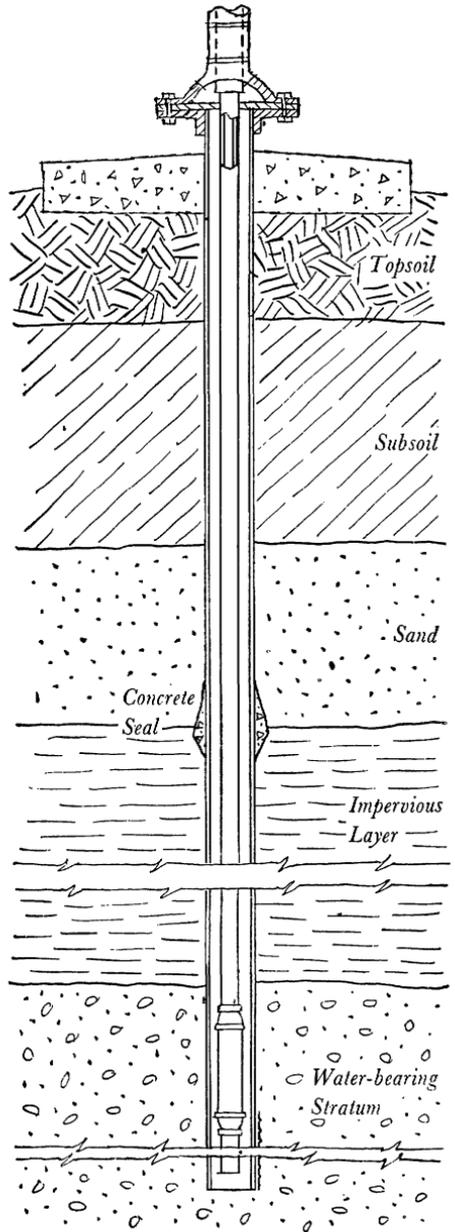
Well drilled through several soil and rock layers, or strata, into water-bearing sand and gravel. Seal is shown at top of impervious layer; also concrete platform at top of well and method of attaching pump to casing.
