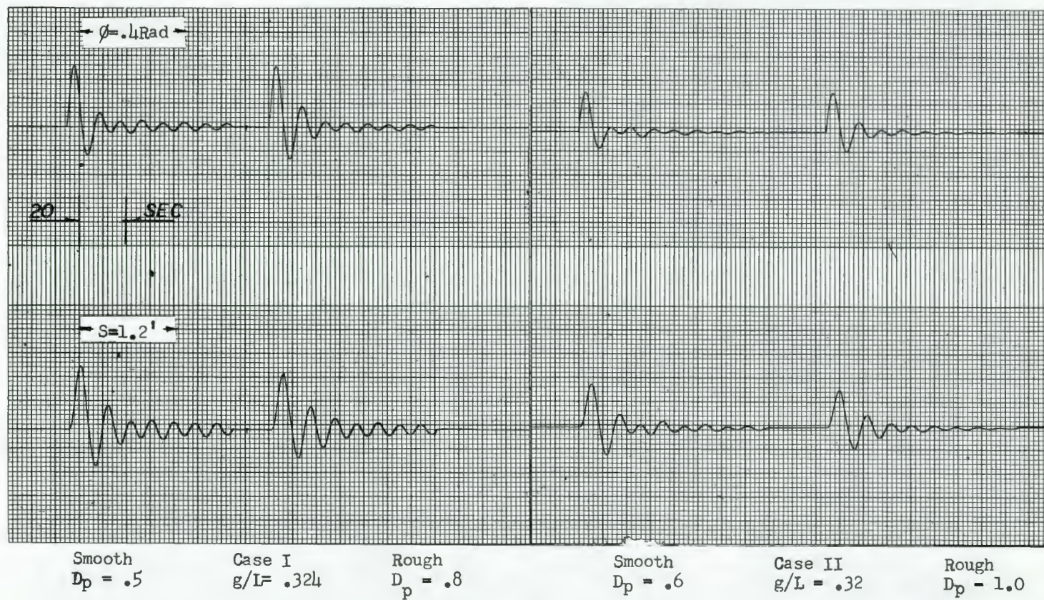
FIGURE X Effect of pipe roughness.
