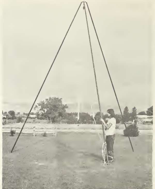
Figure 2.—Tripod mount equipped with 21-foot-long, 1½-inch pipe legs and block and tackle.
