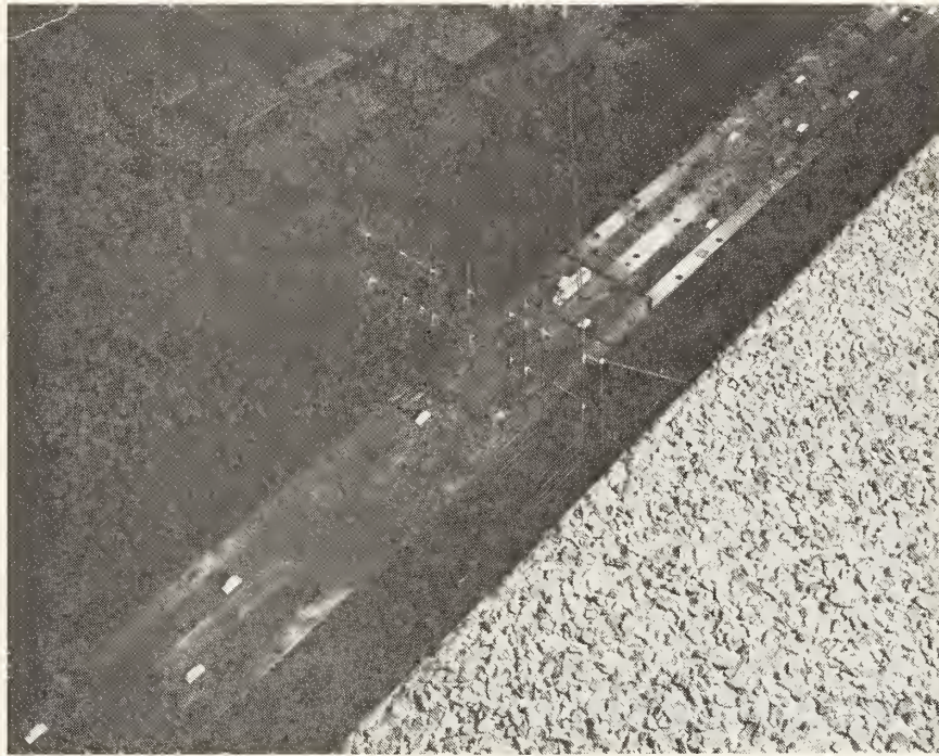
FIGURE 6 CLOSE-UP PHOTO OF THE MODEL SHOWING LARGE AND SMALL ROUGHNESS GROUNDS AND THE GAS-SAMPLING PROBE ARRAY (The Scale of the 0.60-in. Long Cars is 1:300)
