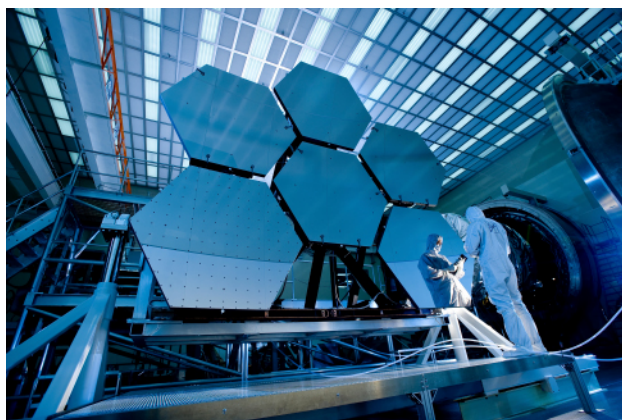
Figure 6.27 James Webb Space Telescope (JWST). This image shows some of the mirrors of the JWST as they underwent cryogenic testing. The mirrors were exposed to extreme temperatures in order to gather accurate measurements on changes in their shape as they heated and cooled. (credit: NASA/MSFC/David Higginbotham/Emmett Given)
