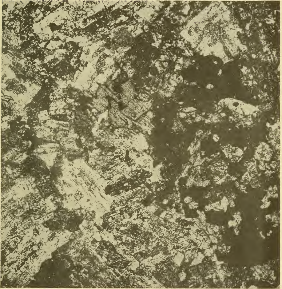
FIG. 2.—Photomicrograph of Amherst sandstone. Polarized light; nicols crossed; magnification 35 \times .
