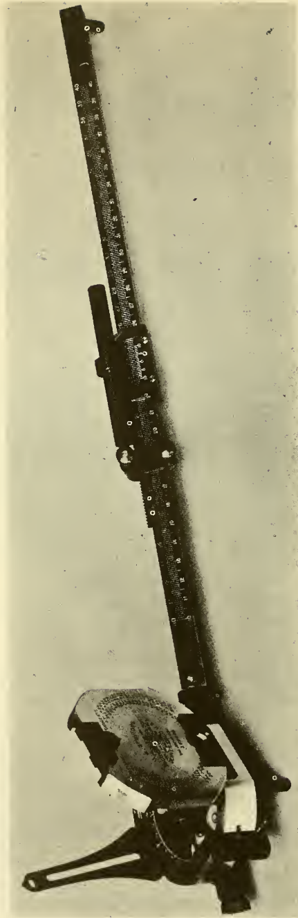
FIG. 1.—Brunton compass attachment for measurement of horizontal magnetic intensity.
