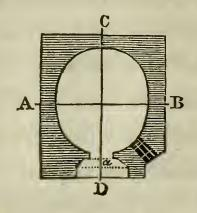
A piece of cast iron covers the space before the door of the oven, exactly level with its floor; the opening underneath is applied to no particular use, but is generally made a receptacle for coal.
