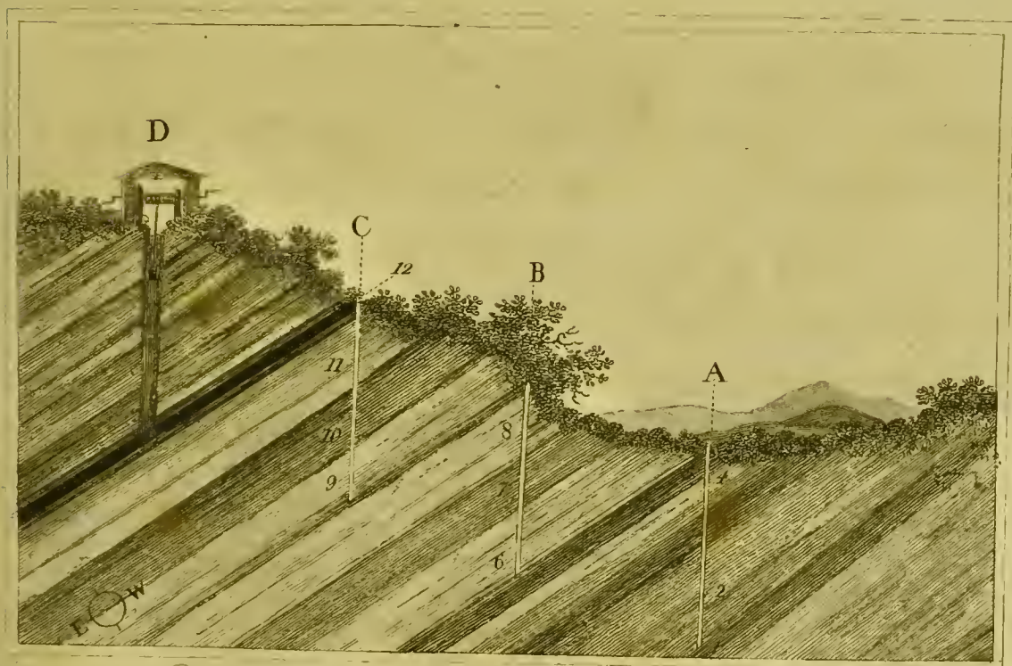
Plan illustrating the method of boring for Coal
