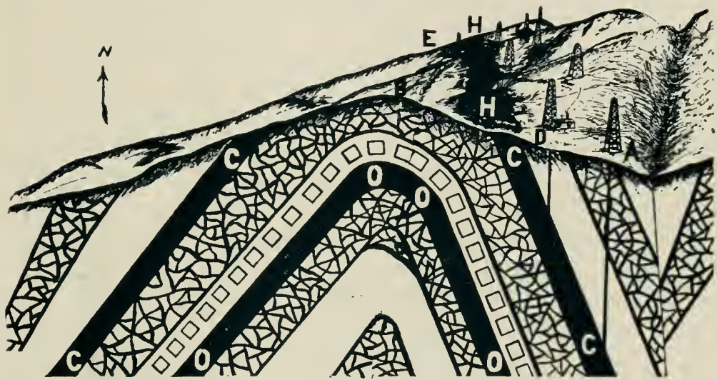
Ideal section of oil field on anticlinal fold; oil-line developed on one limb of the fold.
