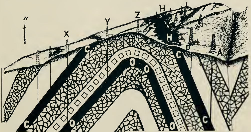
Ideal section of oil-field on anticlinal fold; oil-line developed on both sides of fold.
