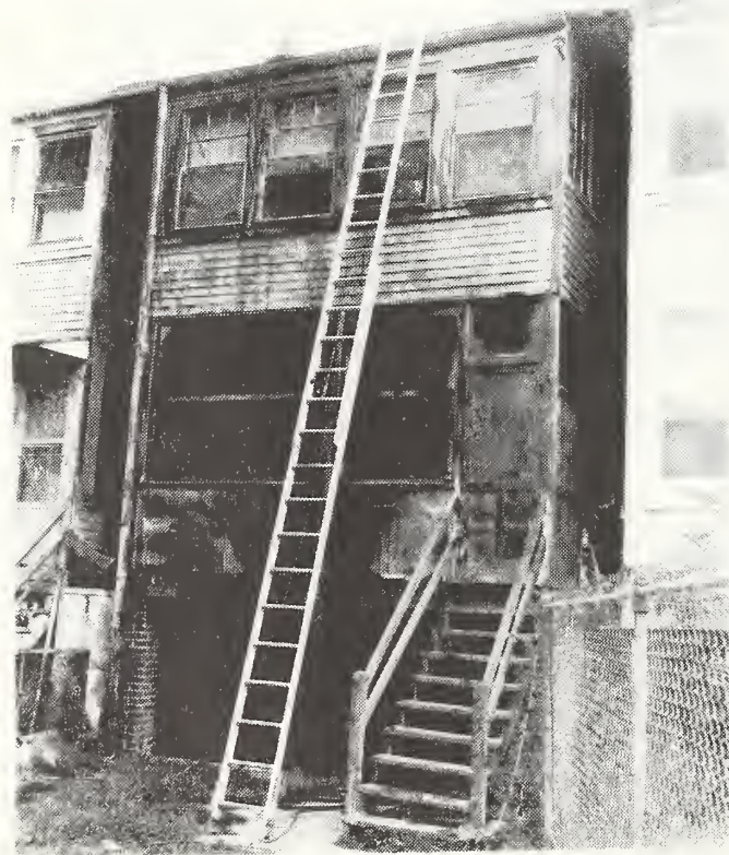
Figure 8. Appearance of paint on wood siding and trim on first floor and basement areas and on metal siding below second floor windows after 30 minutes dwell time of paint remover.
