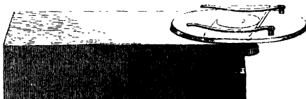
Shadbolt's Turn-table for making Cement-Cells.
