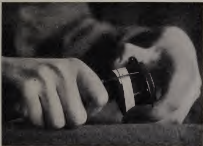
FIG. 57. CUTTING A SLIP OF PAPER TO FIT A LENS
