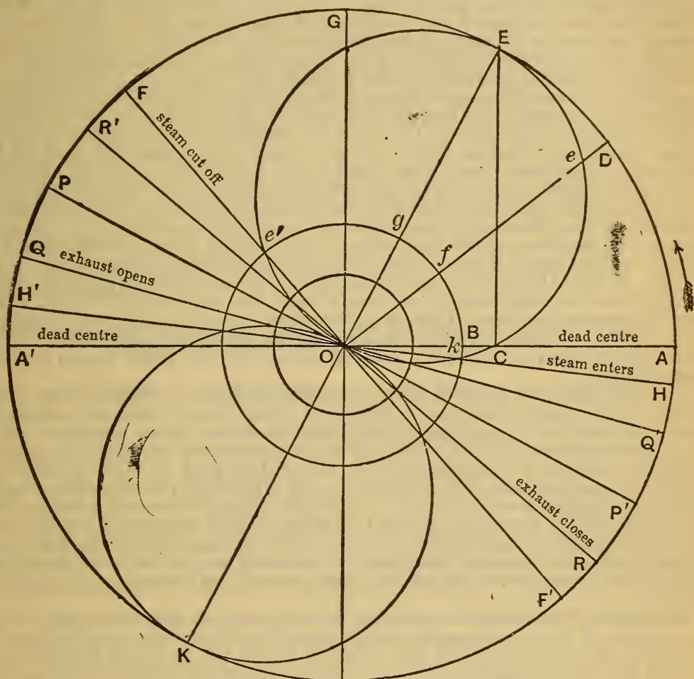
FIG. 148.—Zeuner's Valve-diagram.
