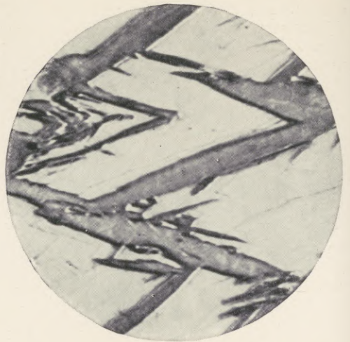
FIG. 2.—Steel containing 1.2 per cent. of carbon quenched in iced brine from a temperature of 1000° C. Mag. 1000 diams.
