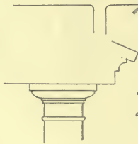
Profile Porch Cornice
