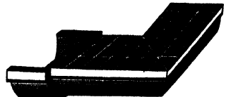
CORNER JUNCTION OF BARTON'S STABLE-DRAINS
