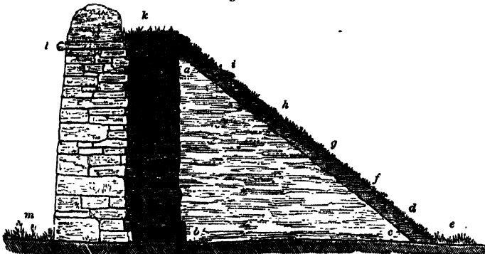
EMBANKMENT AND FACE-DYKE AGAINST A RIVULET.
