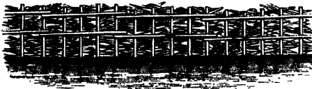
COMMON PILING FOR THE PROTECTION OF RIVER BANKS.
