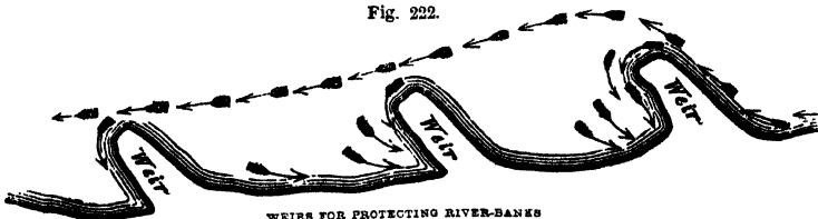
WEIRS FOR PROTECTING RIVER-BANKS
