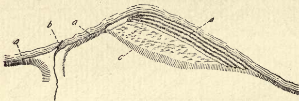
FIG. 22.—South side of The Narrows, Lake Geneva: a, Actively cutting cliffs; b, Mouth of stream turned eastward, showing the prevailing direction of shore drift; c, Steep slope marking original shore line; d, Wave-built terrace.
