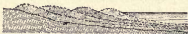
FIG. 19.—Ideal section of a wave-built terrace, built of assorted shore drift. (See p. 28.)
