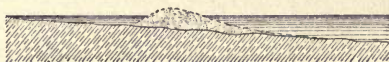
FIG. 17.—Ideal section of a barrier (Gilbert), showing how the offshore slope is steepened by this feature.
