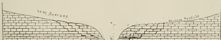
Fig. 1. Diagrammatic illustration of incipient subterranean drainage. The main stream is entrenched and the tributaries out of adjustment pitch over rapids to join it. Underground drainage has started through the joints. The vertical dotted line a b represents the original unbalanced static water head which started the circulation.
