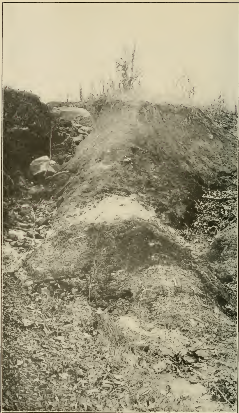
Fig. 1. Outcrop of mahogany clay with white kaolin at top. Sandstone above and shale below. Coal blossom just below note book and below mahogany.
