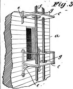
floors or staging from the root to the ground; g g are eircular openings which alternate from one side to the other at each succeeding landing. The landing to be placed before a window at every story.
