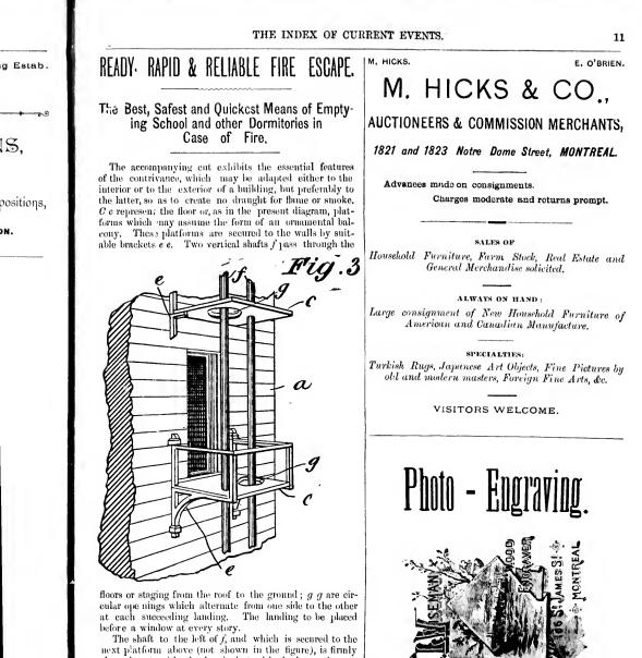
next platform above (not shown in the figure), is firmly clasped, not with the hands, but with the legsand arms, and the person slides down the shaft to the next landing below, regulating with case, by the pressure of his limbs, the rapidity of the descent.
