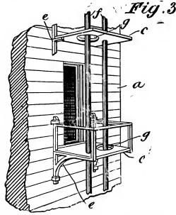
floors or staging from the norm to the ground; g g are circular openings which alternate from one side to the other at each subsecting handing. The landing to be placed before a window at every story.
