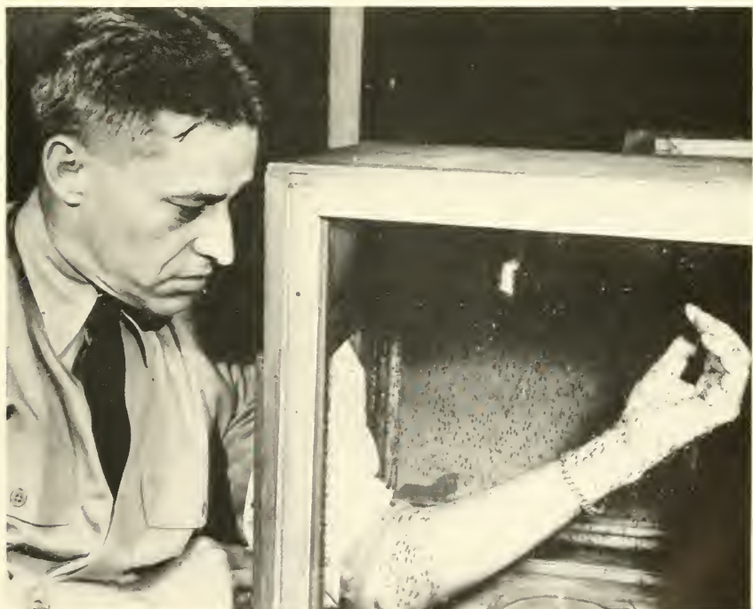
2. Laboratory test of insect repellent. Candidate insect repellents were first tested in the laboratory using caged mosquitoes. Here Dr. B. V. Travis has inserted his partially treated arm in a cage containing several thousand hungry mosquitoes.
