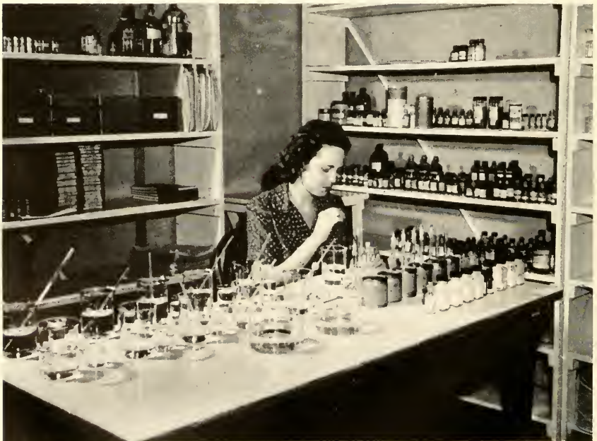
2. A scene in the larvicide testing room. Edna Hinchey is shown adding the desired concentration of a test chemical to water in a beaker prior to introduction of mosquito larvae.
