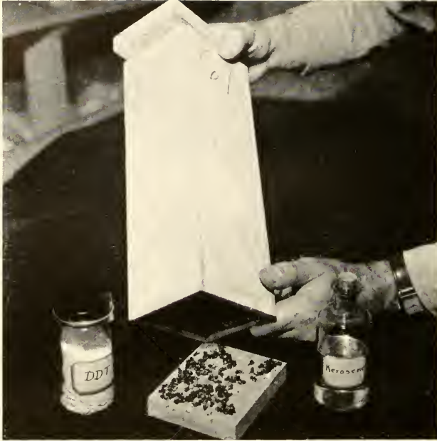
One type of cage employed in conducting DDT laboratory tests. Various concentrations of DDT employing different kinds of formulations were tested as a residual treatment to determine the duration of effectiveness against mosquitoes and flies.
