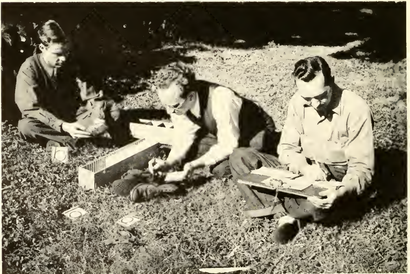
2. Testing miticides. Several thousand candidate materials were tested. The initial test procedures consisted of "stopping time" tests. Here F. M. Snyder (center) and assistants are placing chiggers collected in infested areas on cloth patches treated with miticides to determine if they are effective miticides.
