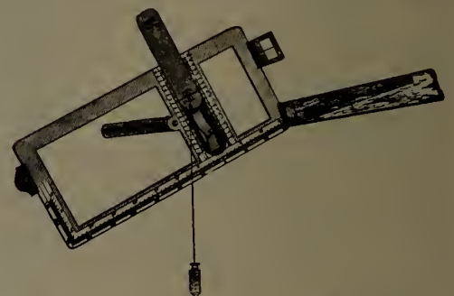
FIG. 3.—FAUSTMANN'S HEIGHT MEASURE.
