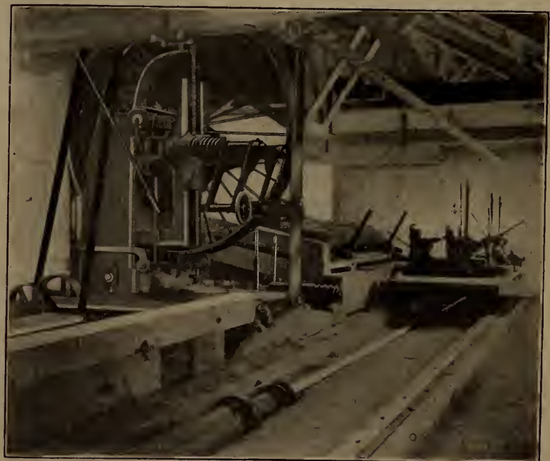
One of the many Double Cutting Band Mills with 8 ft. Band Wheel in Actual Operation
