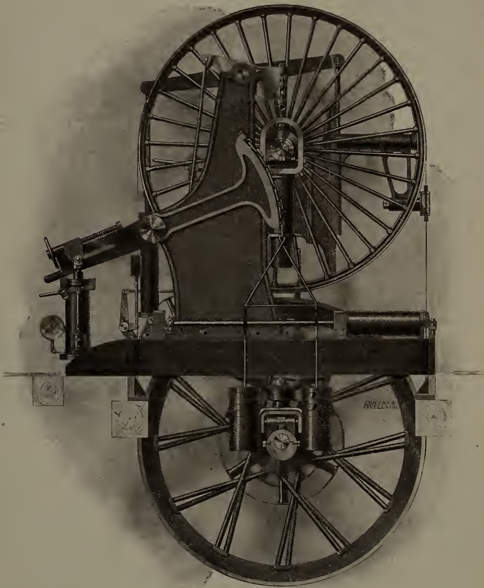
STEAM TENSION BAND MILL MANUFACTURED BY WM. HAMILTON MANUFACTURING CO.
