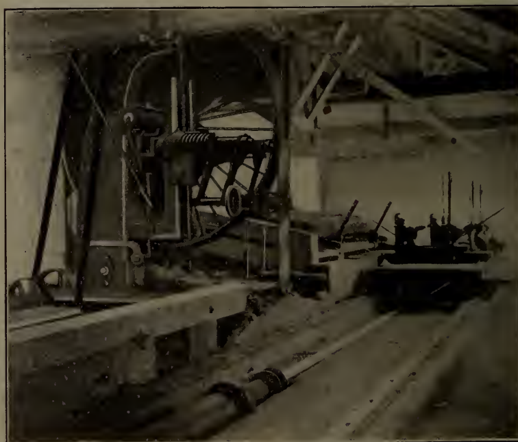
One of the many Double Cutting Band Mills with 8 ft. Band Wheel in Actual Operation
