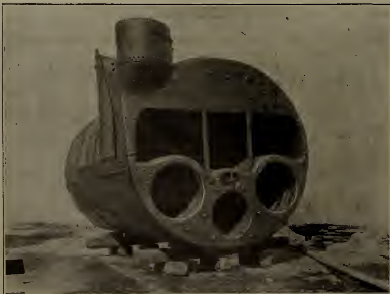
One of two Marine Boilers built in our shops for the Richelieu & Ontario Navigation Co's Steamer 'Carolina.' Length 21' 4", diameter 13' 4", height 11' 10", weight 37½ tons.
