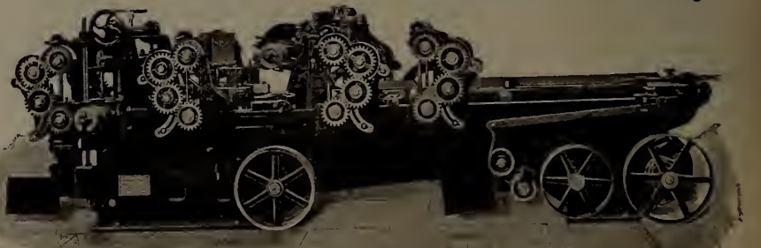
Heavy 25 inch Divided Roll Planer and Matcher with 8 Feed Rolls.
