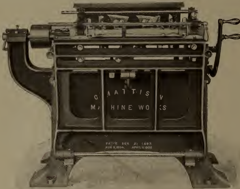
BALUSTER TURNING LATHE MANUFACTURED BY C. MATTISON MACHINE WORKS.
