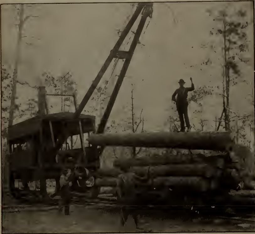
MISSISSIPPI : A "MCGIFFERT" LOADER IN THE SOUTH HANDLING LONG ONES. Note the manner in which it permits empty cars to pass under or through itself.
