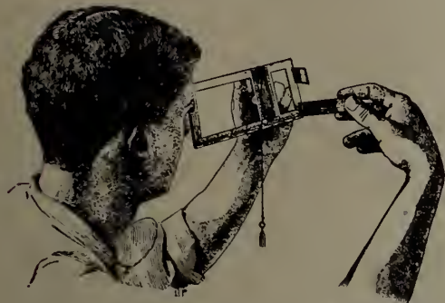
FIG. 4.—MANNER OF USING FAUSTMANN'S HEIGHT MEASURE.
