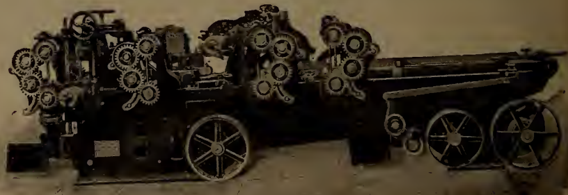
Heavy 26 inch Divided Roll Planer and Matcher with 8 Feed Roll.
