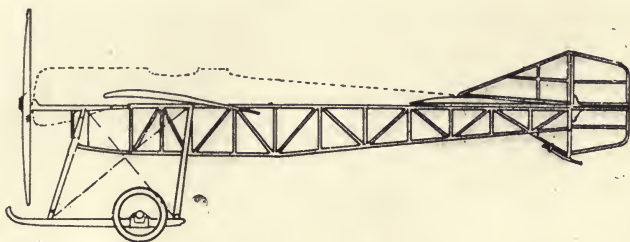
FIG. 48.—RIGID TYPE OF GIRDER FUSELAGE.
